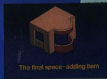
The 3-D cladding element is clipped on
