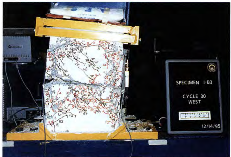
Fig. 15. Typical test specimen with fiber reinforced concrete (University of Michigan).
