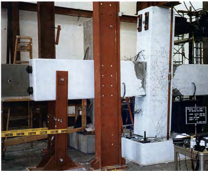
(a) General view of test unit after 5 percent drift
