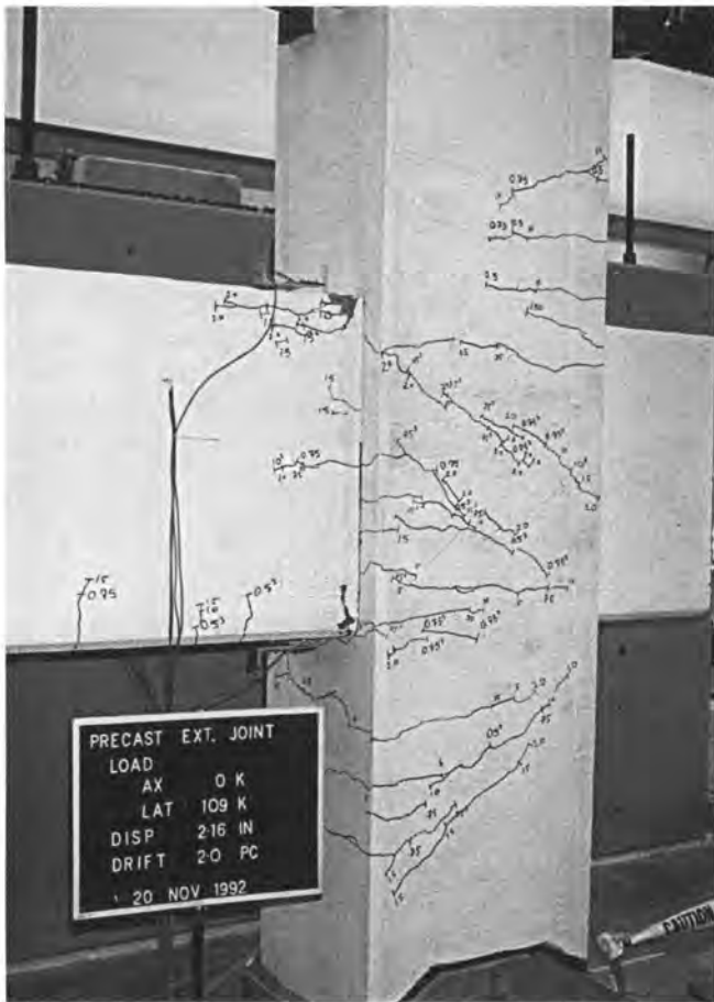
Fig. 7a. Exterior subassembly crack patterns at design and maximum drift. Design drift = 2 percent.
