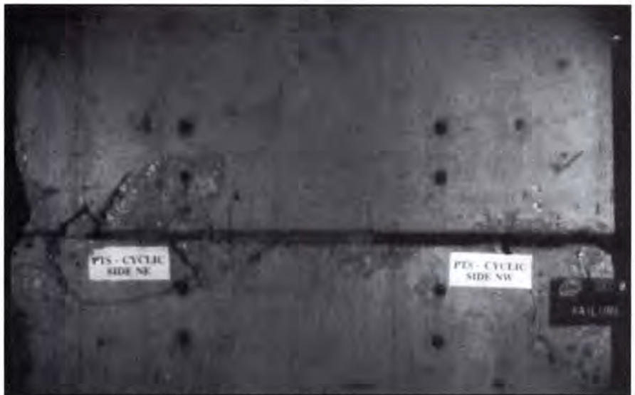
Fig. 5(a). Failure modes for Connection PTS.
