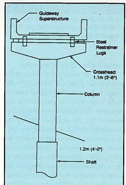
Fig. 8. Typical guideway substructure.
