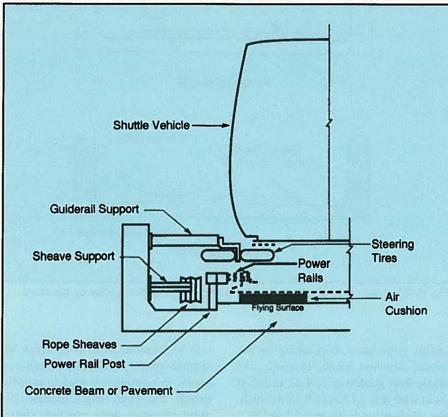
Fig. 5. The guideway/vehicle system interfaces.
