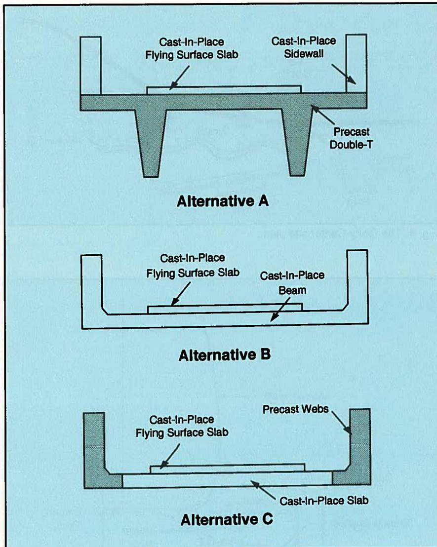
Fig. 6. Alternate cross sections considered in designing the guideway structure.
