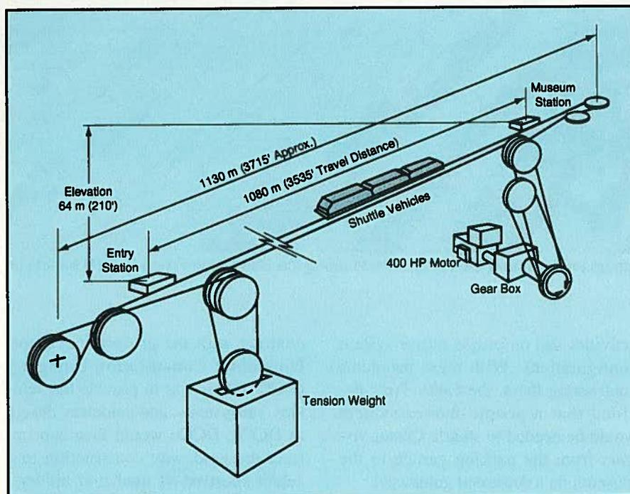
Fig. 3. Schematic of the cable drive system.
