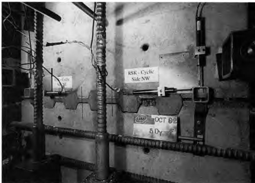
Fig. 7(b). Failure mode for Specimen RSK.
