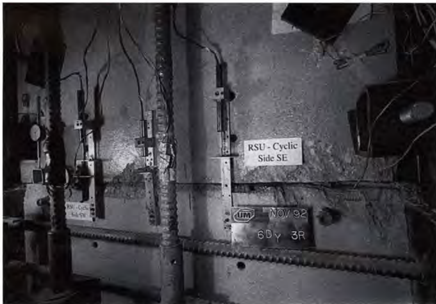
Fig. 7(a). Failure mode for Specimen RSU.
