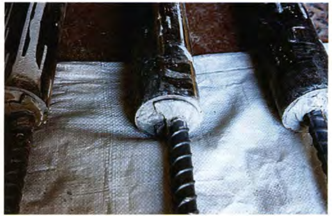
Fig. 7. Splitting failure, Type 1 specimen.
