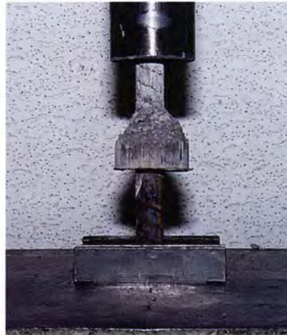
Fig. 9. Typical bond failure for Type 3 specimens.
