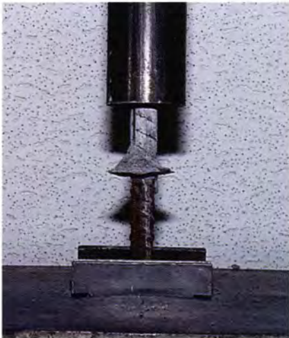
Fig. 8. Typical bond failure for Type 2 specimens.
