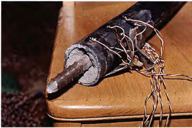
Fig. 6. Tensile strength failure, Type 3, Specimen 5.
