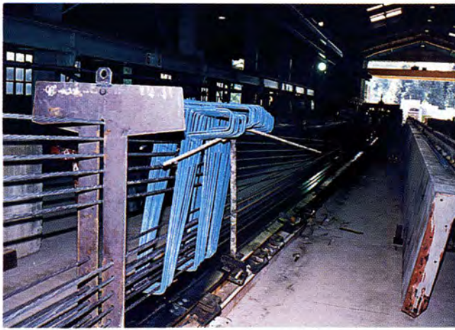
Fig. 11. Prestensioned T-girder; shear reinforcement is epoxy coated.
