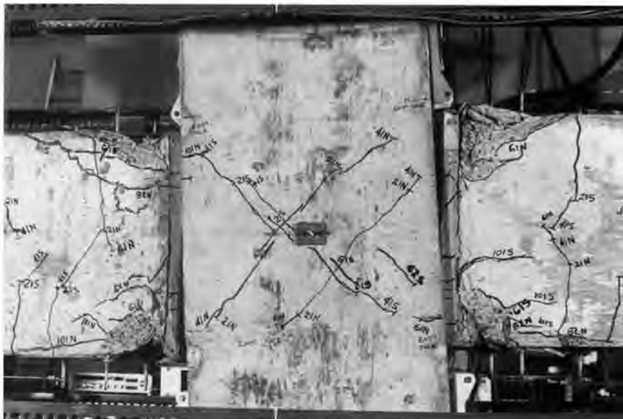
Fig. 23. Representative failure mode for the precast concrete specimens.
