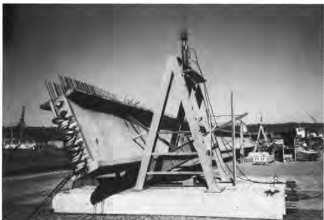
Fig. 6. Test beam near maximum tilt of 32 degrees.
