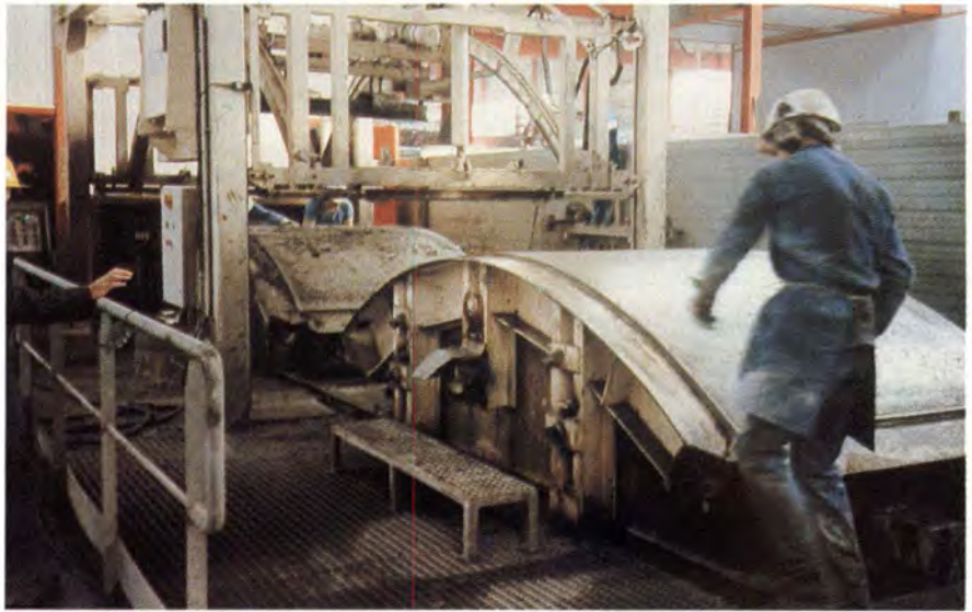
Fig. 1. Highly impermeable concrete with a water-cement ratio of 0.32 for Eurotunnel tunnel liners.
