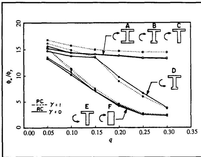
Fig. 8. Effect of section shape on the ductility factor.
