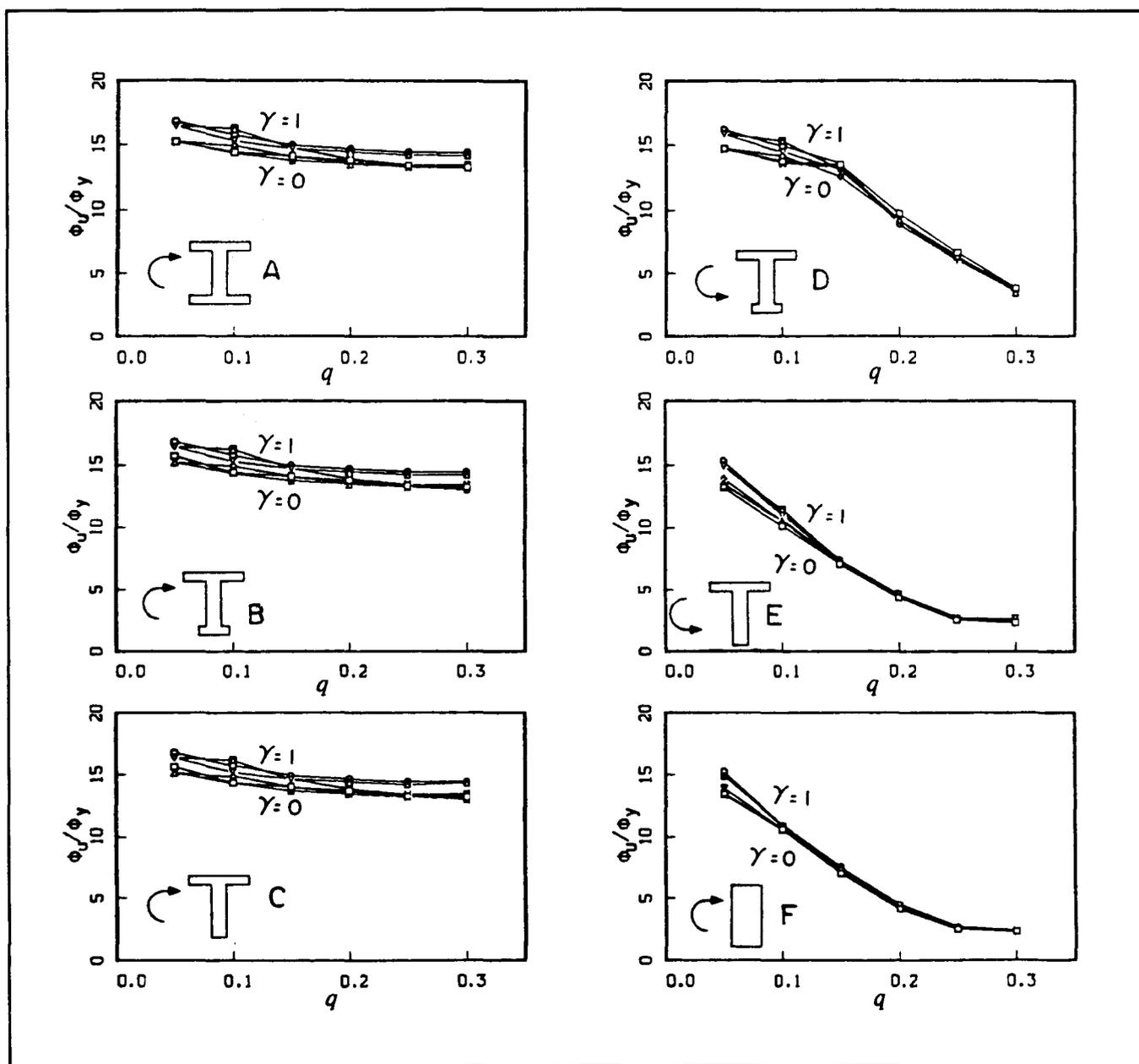
Fig. 7. Effect of mixed reinforcement index on the ductility factor vs. mechanical steel percentage relationship.
