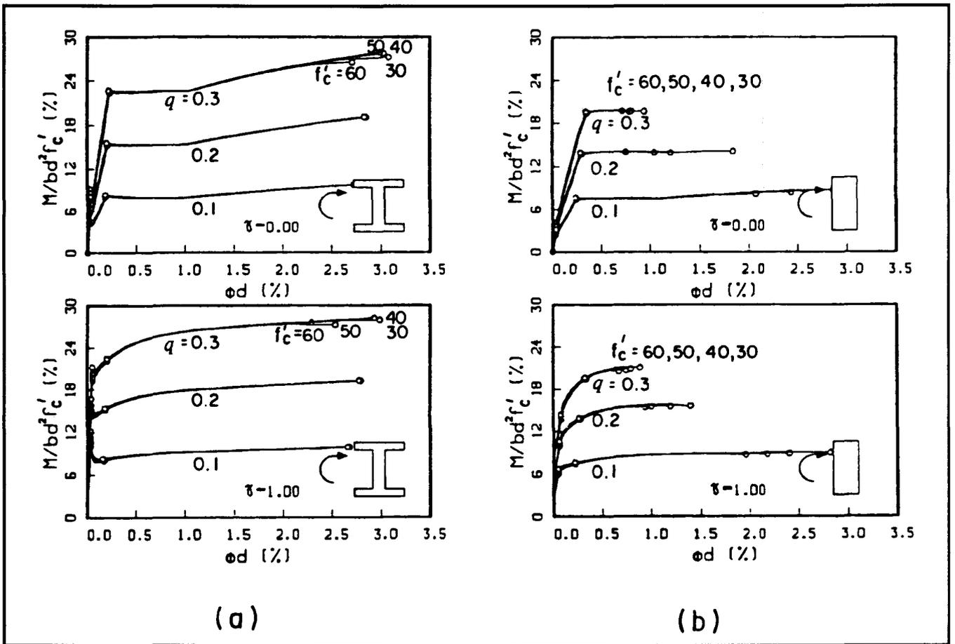
Fig. 12. Effect of concrete grade on the moment-curvature relationship: (a) I-section; (b) rectangular section.
