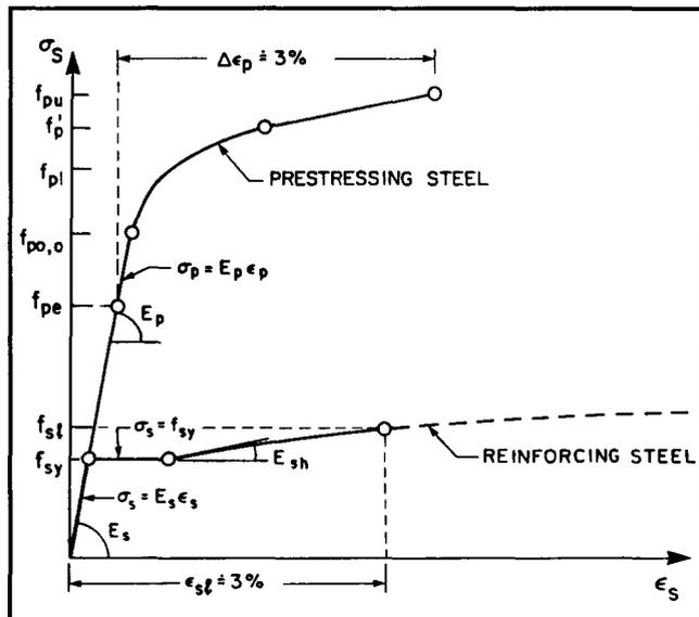
Fig. 3. Constitutive laws for reinforcing steel (nonprestressed) and prestressing steel.<sup>7</sup>
