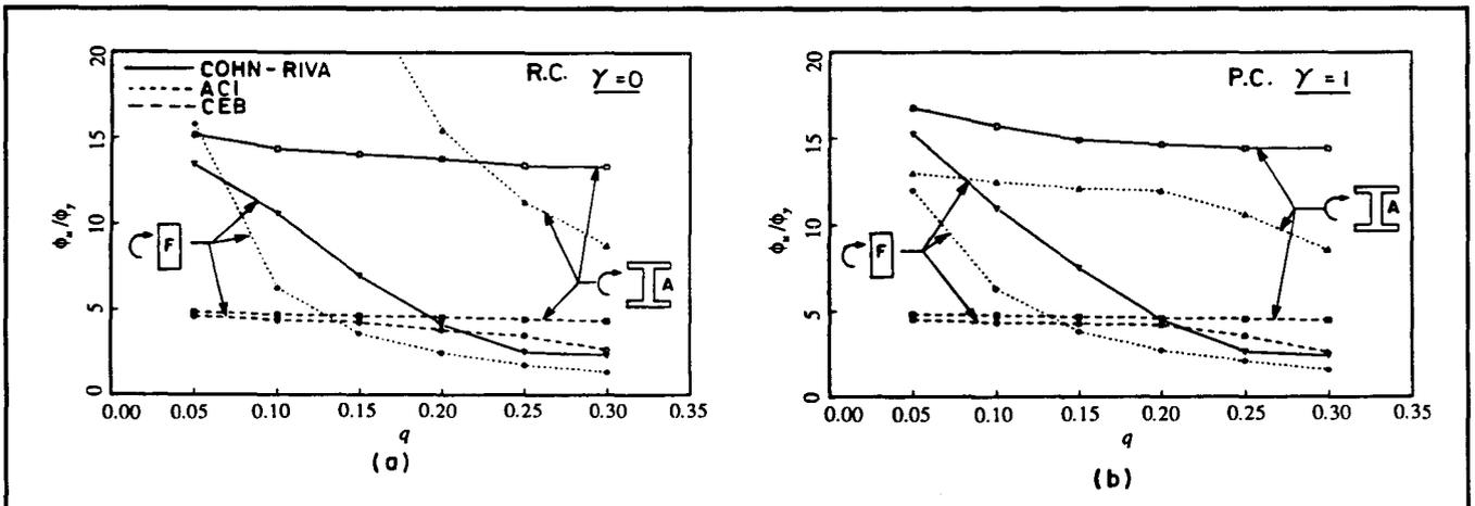
Fig. 11. Ductility factor vs. reinforcement index relationships according to models by Cohn-Riva, ACI and CEB codes: (a) RC sections; (b) PC sections.
