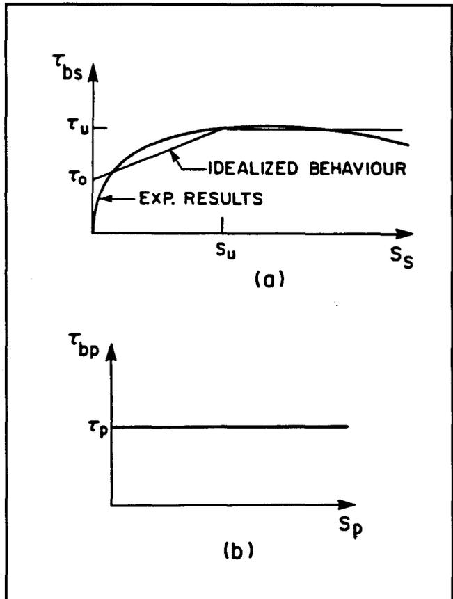
Fig. 4. Bond-slip constitutive relations:<sup>17</sup> (a) reinforcing steel; (b) prestressing steel.
