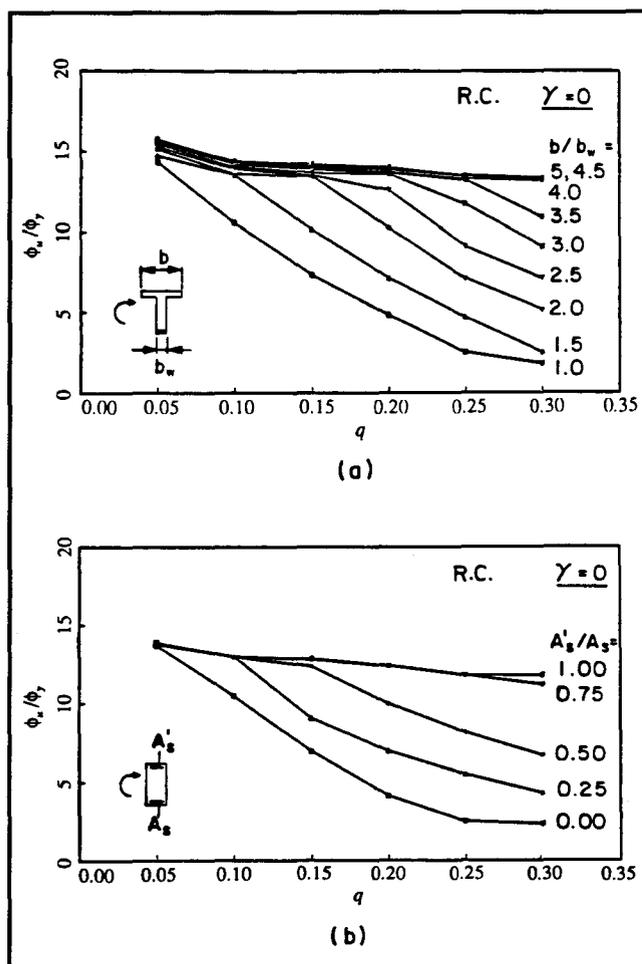
Fig. 9. Ductility factor vs. reinforcement index variation for RC and PC sections: (a) effect of flange to web width ratio; (b) effect of compression reinforcement.
