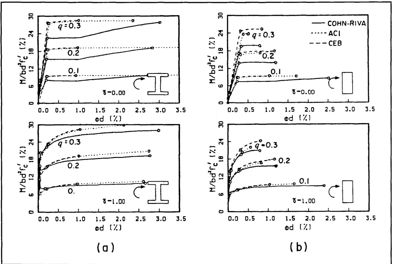
Fig. 10. Moment-curvature relationships according to models by Cohn-Riva, ACI and CEB codes: (a) I-section; (b) rectangular section.
