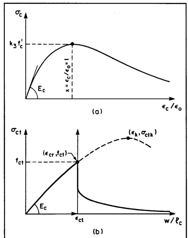
Fig. 2. Constitutive laws for concrete: (a) compression;<sup>7</sup> (b) tension.<sup>18</sup>
