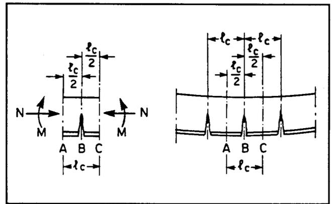
Fig. 1. Typical element for which the local moment-curvature law is studied.
