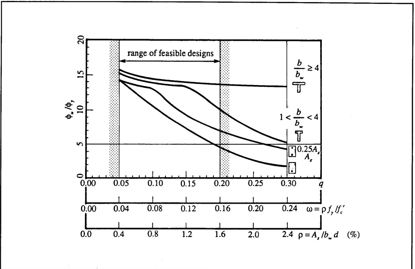
Fig. 15. Combined effects of section shape and compression reinforcement on the ductility factor [for  $f'_c = 40$  MPa (5.8 ksi) and  $f_y = 400$  MPa (58 ksi)].
