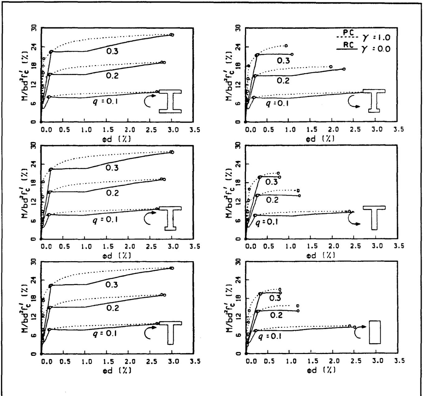
Fig. 5. Effect of section shape on the moment-curvature relationship.
