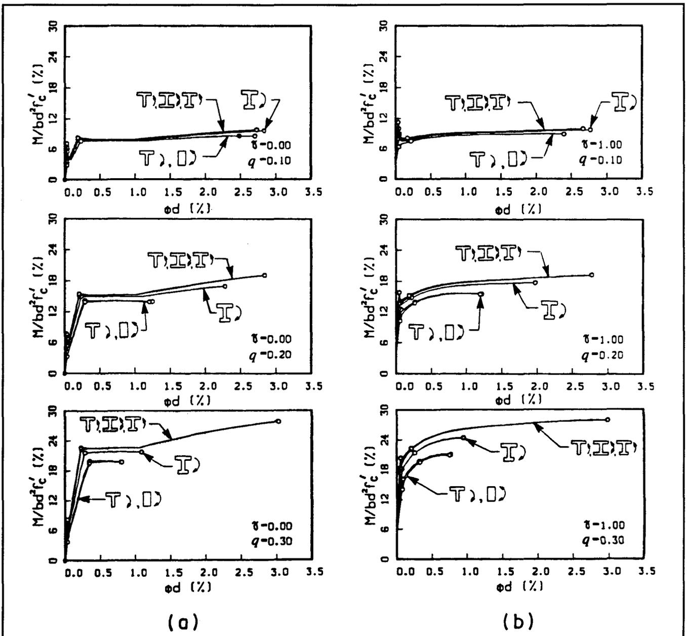
Fig. 6. Effect of section shape on the moment-curvature relationship: (a) reinforced concrete sections; (b) fully prestressed concrete sections.
