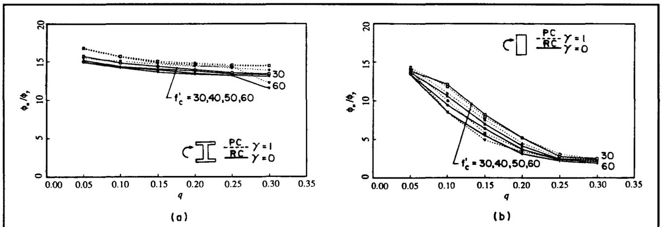
Fig. 13. Effect of concrete grade on concrete and reinforcing steel strains at the ultimate limit state: (a)  $f'_c = 30$  MPa (4.35 ksi); (b)  $f'_c = 60$  MPa (8.70 ksi).
