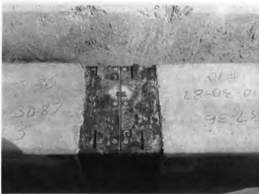
Fig. 8. Tension test specimen at maximum load.
