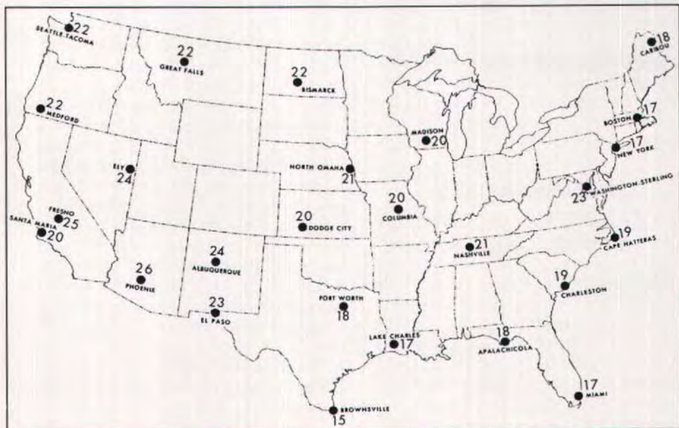
Fig. 4. Computed maximum temperature differences ( ^{\circ}\text{C} ) of 2 m (6.56 ft) deep bridge structures, with 50 mm (2 in.) blacktop, located at different SOLMET stations.
