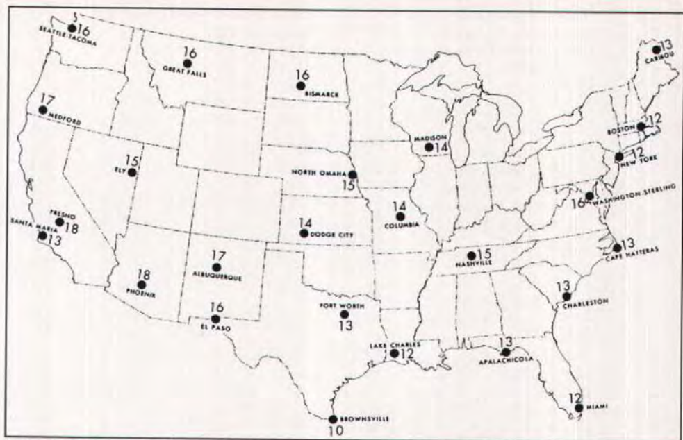
Fig. 5. Computed maximum temperature differences ( ^{\circ}\text{C} ) of 2 m (6.56 ft) deep bridge structures, with 100 mm (4 in.) blacktop, located at different SOLMET stations.
