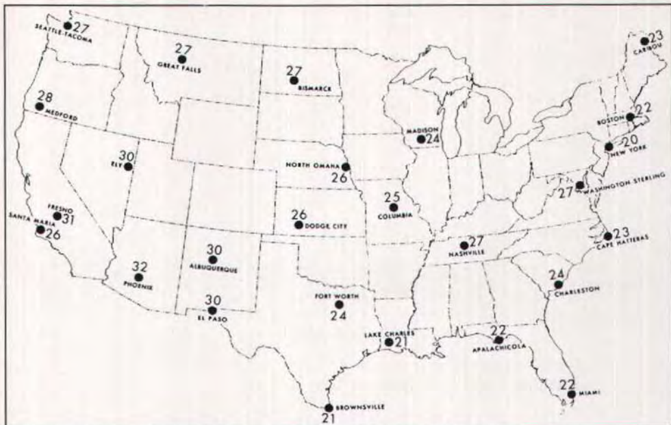
Fig. 3. Computed maximum temperature differences ( ^{\circ}\text{C} ) of 2 m (6.56 ft) deep bridge structures (unsurfaced) located at different SOLMET stations.
