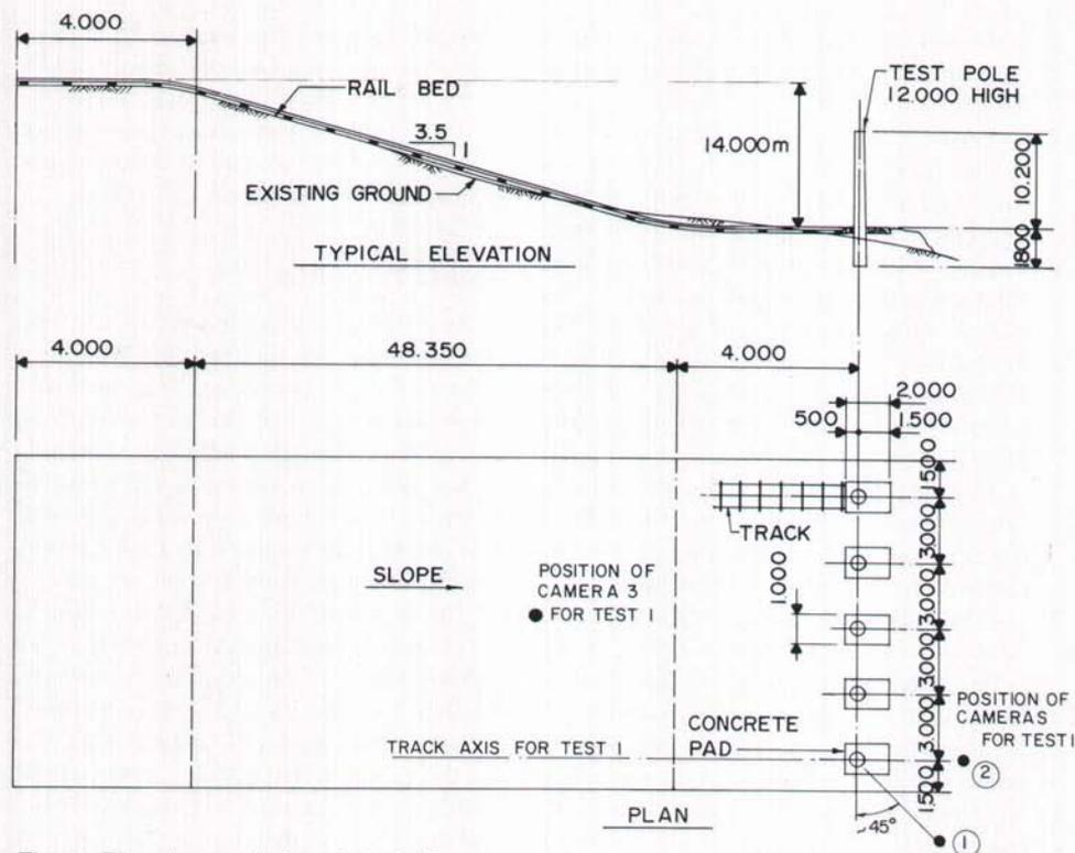
Fig. 3. Elevation and plan of test site.
