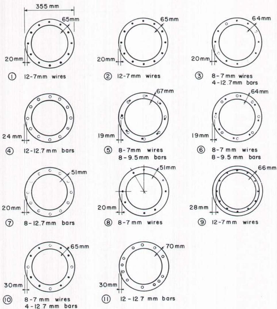
Fig. 2. Cross section of poles at ground level.
