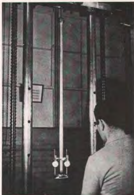
Fig. 12. 50-in. Double Dial extensometer in use.
