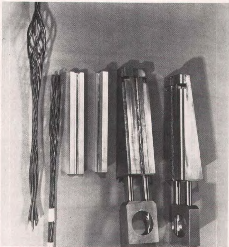
Fig. 7. Tinius Olsen SLS Grips, new liners for grips and strand that broke in clear between grips.
