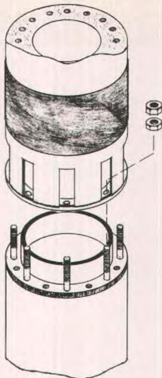
Fig. 40b. Schematic of bolted splice.
