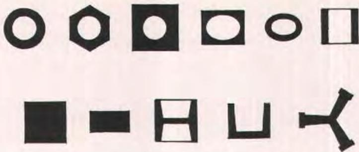
Fig. 22. Typical cross sections of prestressed concrete poles.
