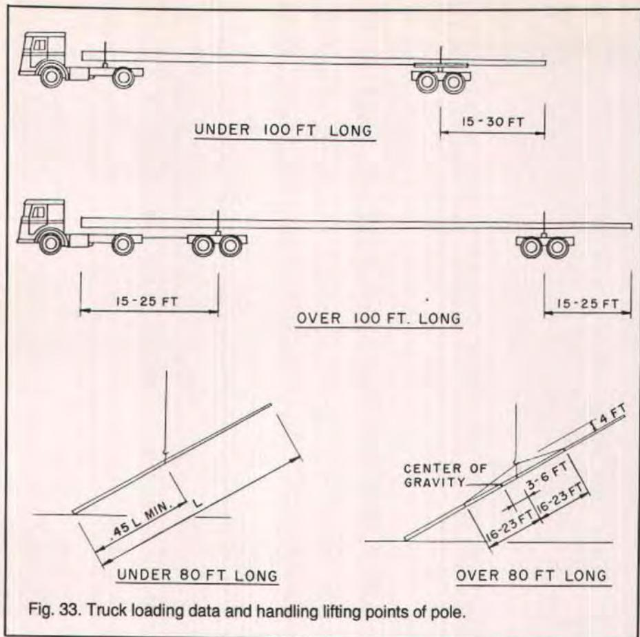
Fig. 33. Truck loading data and handling lifting points of pole.
