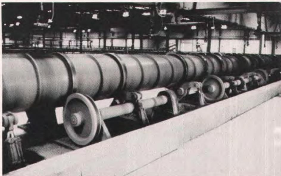
Fig. 26. Pole spinning operation.
