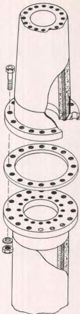
Fig. 42b. Schematic of flange plate splice.
