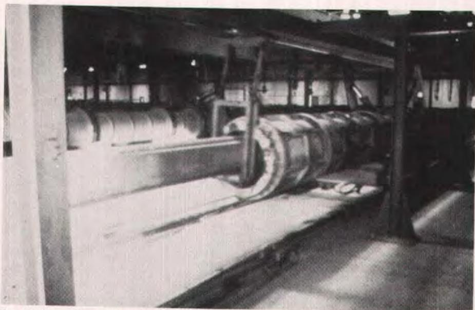
Fig. 24. Closed form concrete placement used in manufacture of poles.
