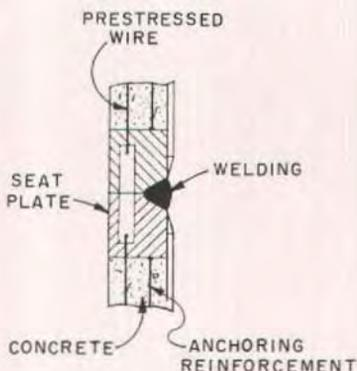
Fig. 39b. Schematic of welded splice (Japanese).
