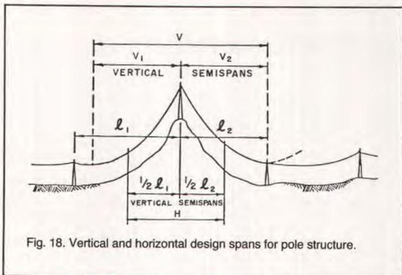
Fig. 18. Vertical and horizontal design spans for pole structure.
