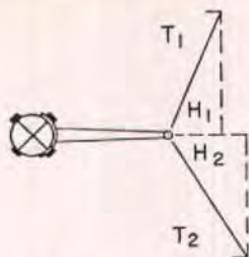
Fig. 20. Line angle loads acting on pole structure. Note:
