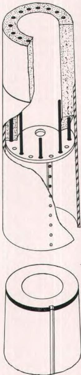
Fig. 41b. Schematic of slip joint splice.
