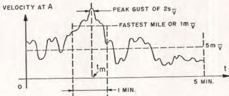
Fig. 19. Wind velocity strip graph for designing pole structure.
