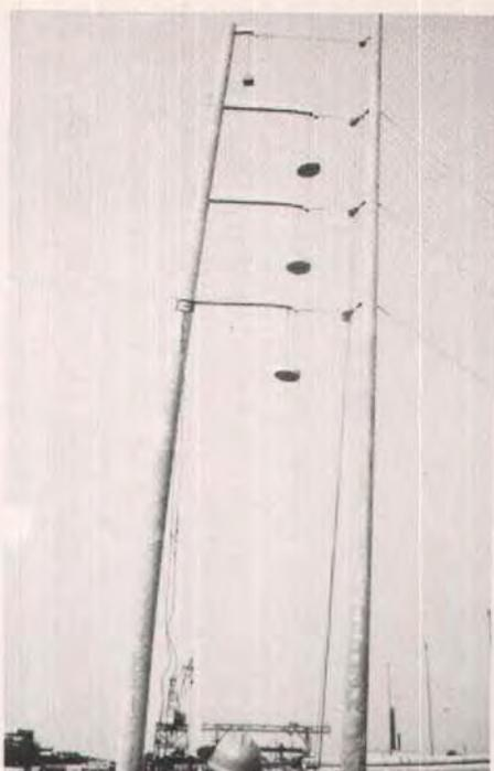
Fig. 29. Structural testing of prestressed concrete pole structure.
