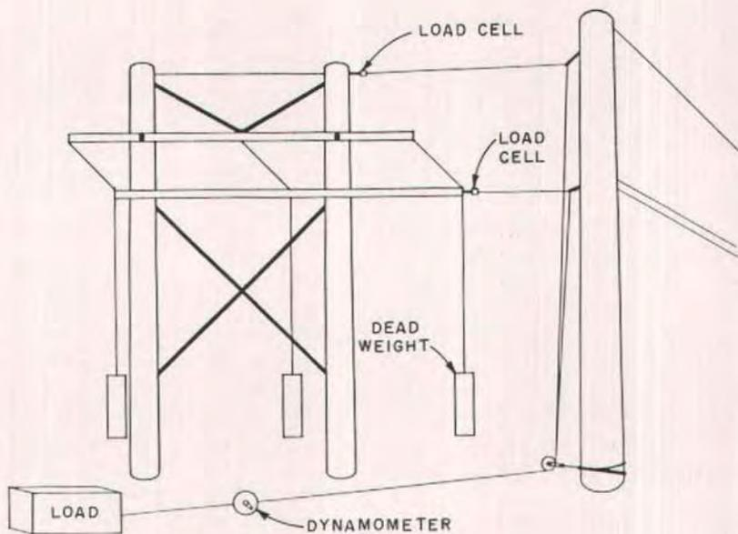
Fig. 32. Equipment used in testing pole structure.
