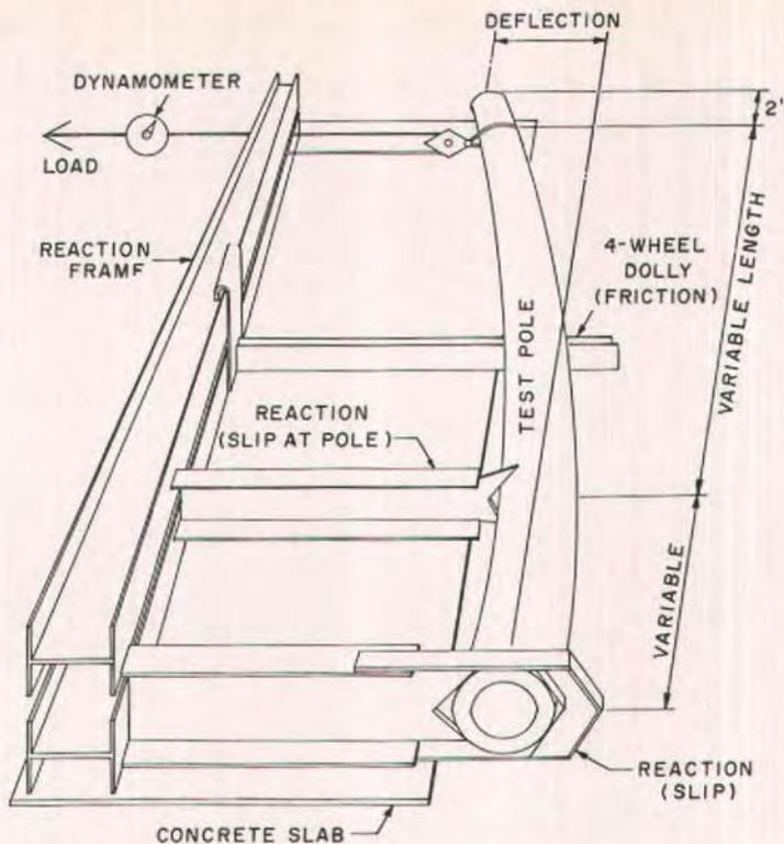
Fig. 31. Schematic of horizontal testing of concrete pole for flexural capacity.
