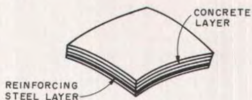
(b) LAYER DISCRETIZATION OF THICKNESS
