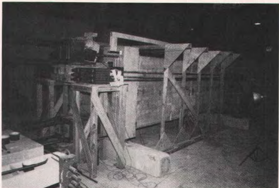
Fig. 28. Load cell arrangement for Specimen 1.
