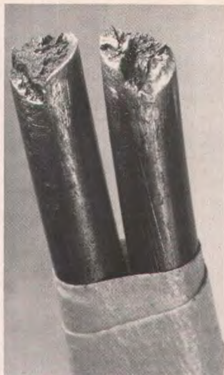
Fig. 1. Typical failure mode without surface attack.
