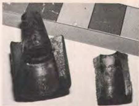
Fig. 7. Failed barrel of 0.6-in. (15 mm) strand anchorage showing longitudinal failure surface.
