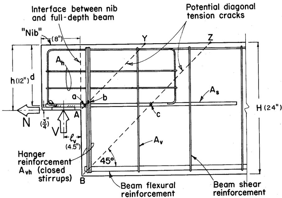
Fig. 2. Typical dapped-end reinforcement and location of potential diagonal tension cracks. Note that the dimensions in parentheses are those of the test specimens.
