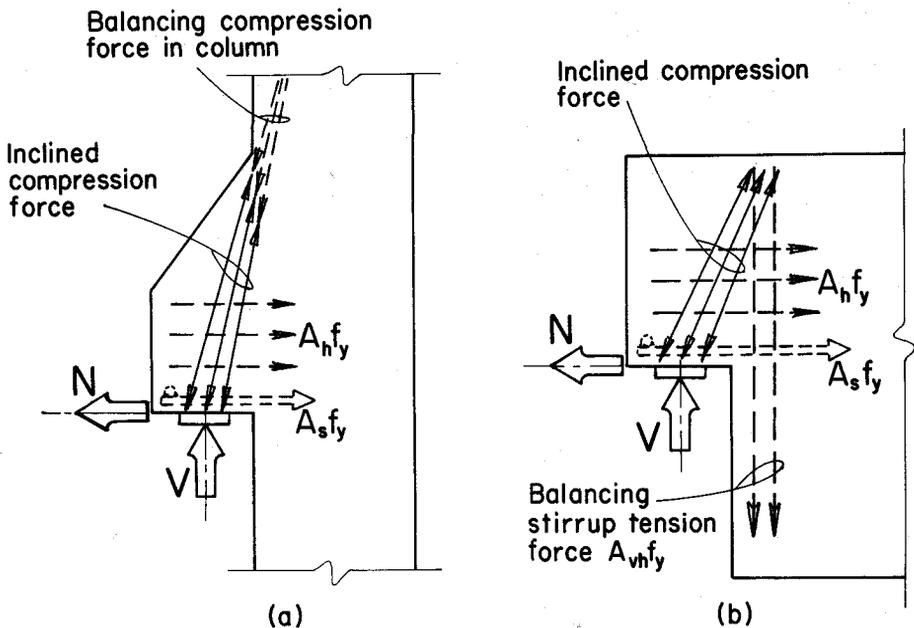
Fig. 1. Comparison of internal force systems: (a) in corbel on a column and (b) in a dapped-end beam.
