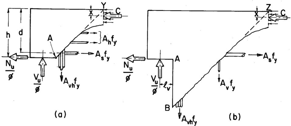
Fig. 3. Forces assumed acting on free bodies cut off by diagonal tension cracks in full-depth beam.
