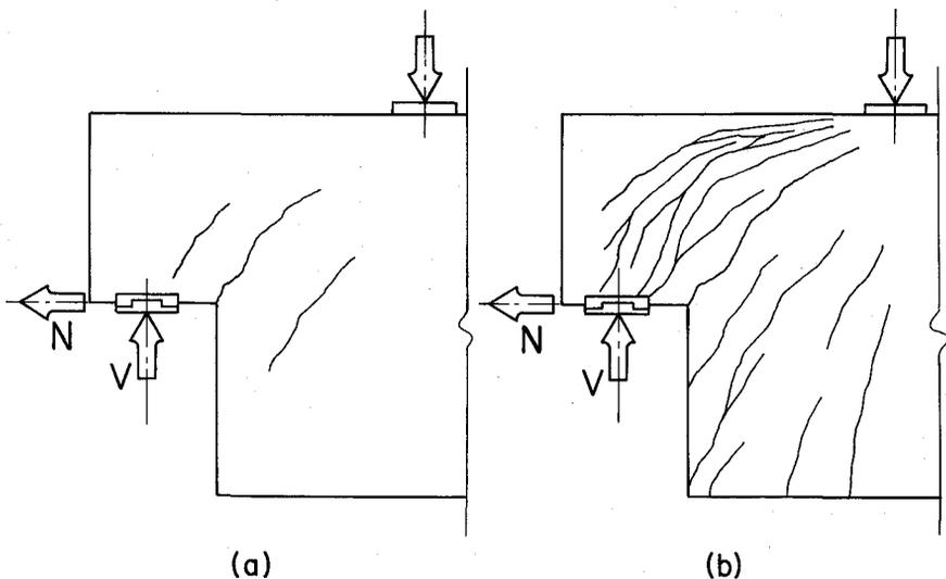
Fig. 6. Typical cracking patterns of dapped-end beams tested: (a) at service load and (b) just before failure.
