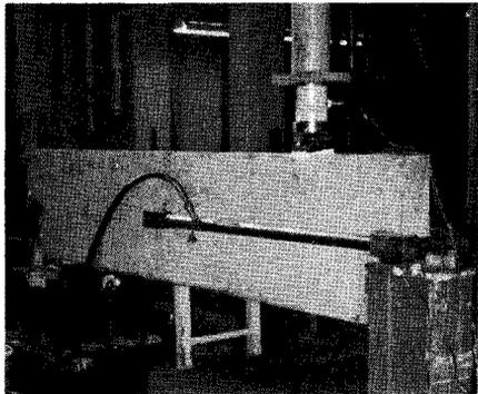
Fig. 5. Test setup in which both horizontal and vertical loads are acting on dapped-end beam.
