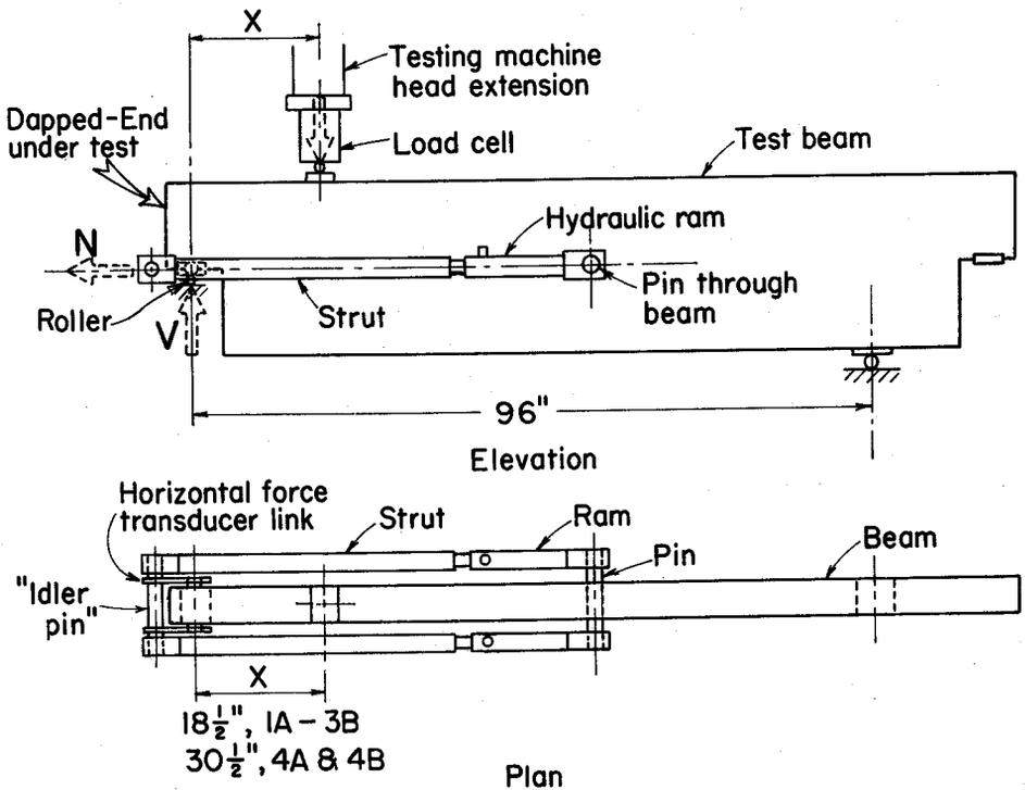
Fig. 4. Testing arrangements for dapped-end beam.
