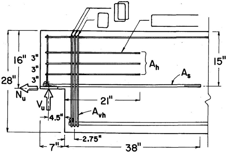
Fig. 7. Design example for dapped-end beam.
