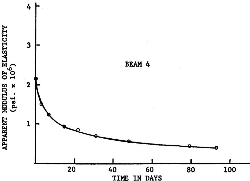
FIG. 9 - APPARENT MODULUS OF ELASTICITY, BEAMS 3 AND 4
