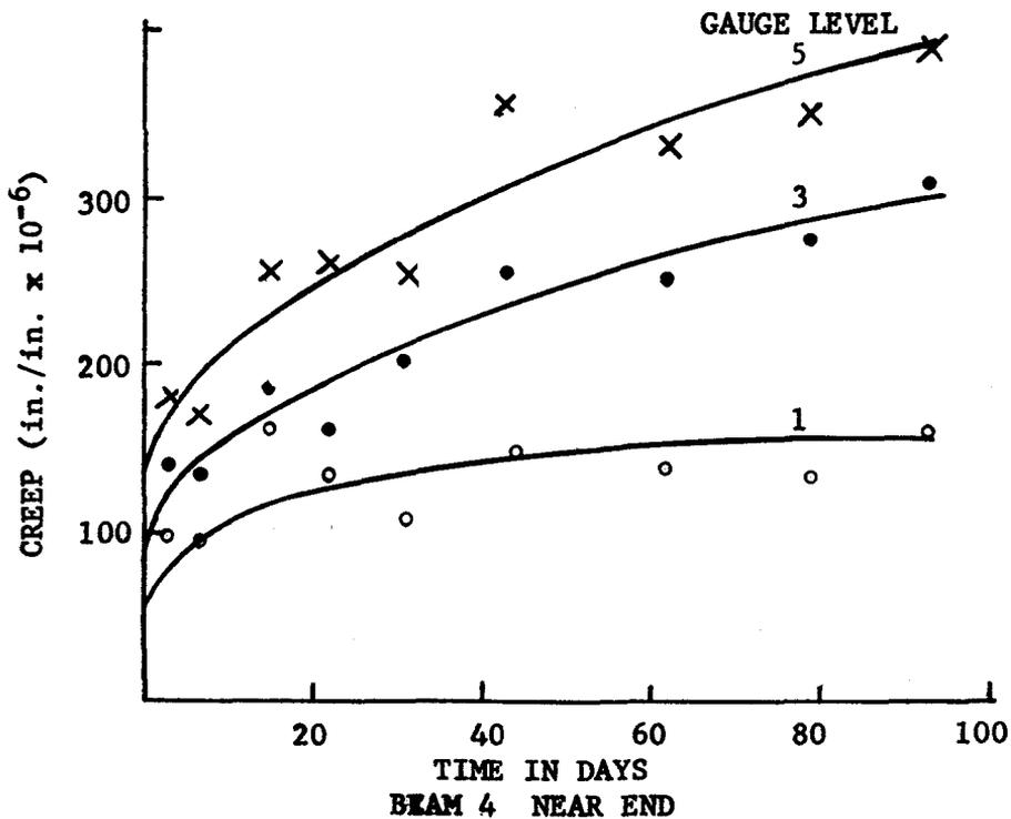
FIG. 18 - CONCRETE CREEP CURVES, BEAMS 3 AND 4
