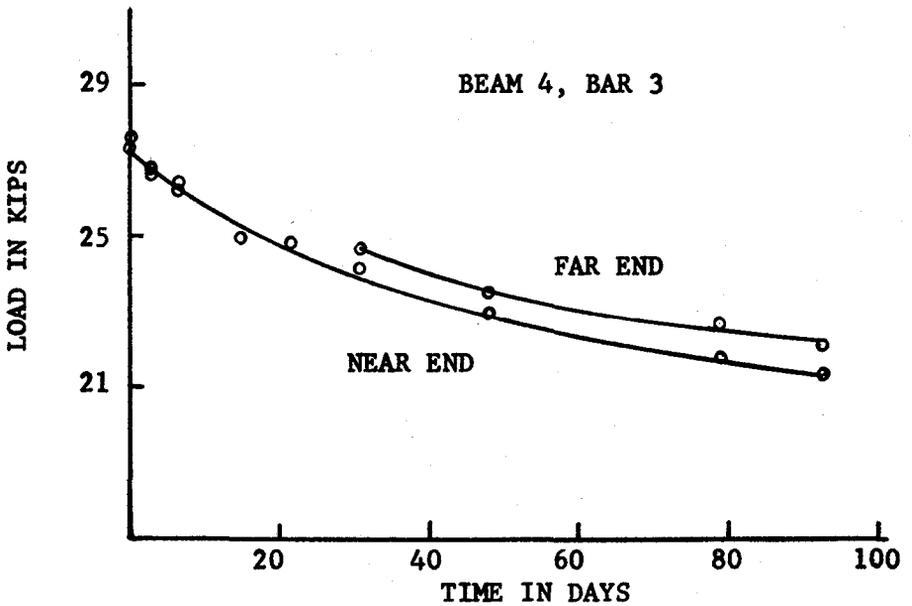
**FIG. 7 - POST-TENSIONING FORCES, BEAM 4**
