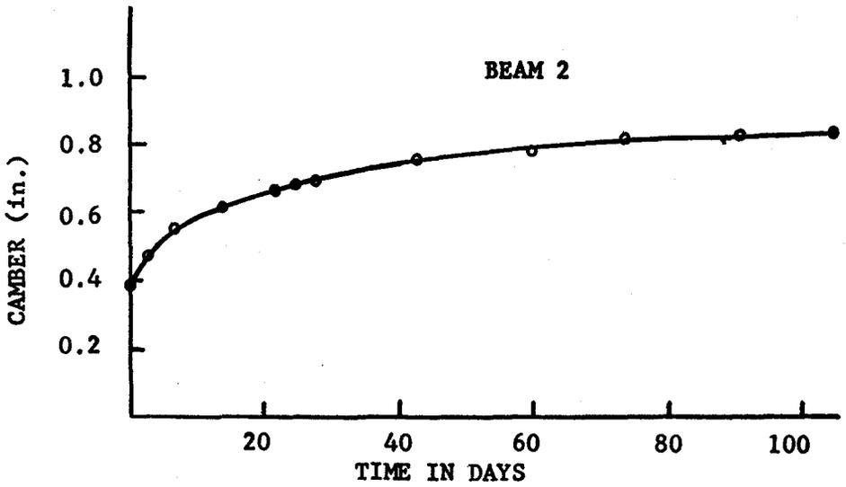
FIG. 3 - CAMBER CURVES, BEAMS 1 AND 2
