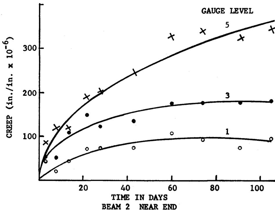
FIG 15 - CONCRETE CREEP CURVES, BEAMS 1 AND 2
