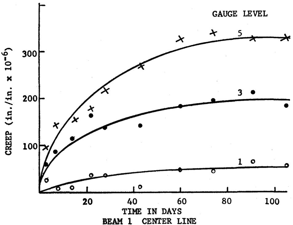
FIG. 14 - CONCRETE CREEP CURVES, BEAM 1
