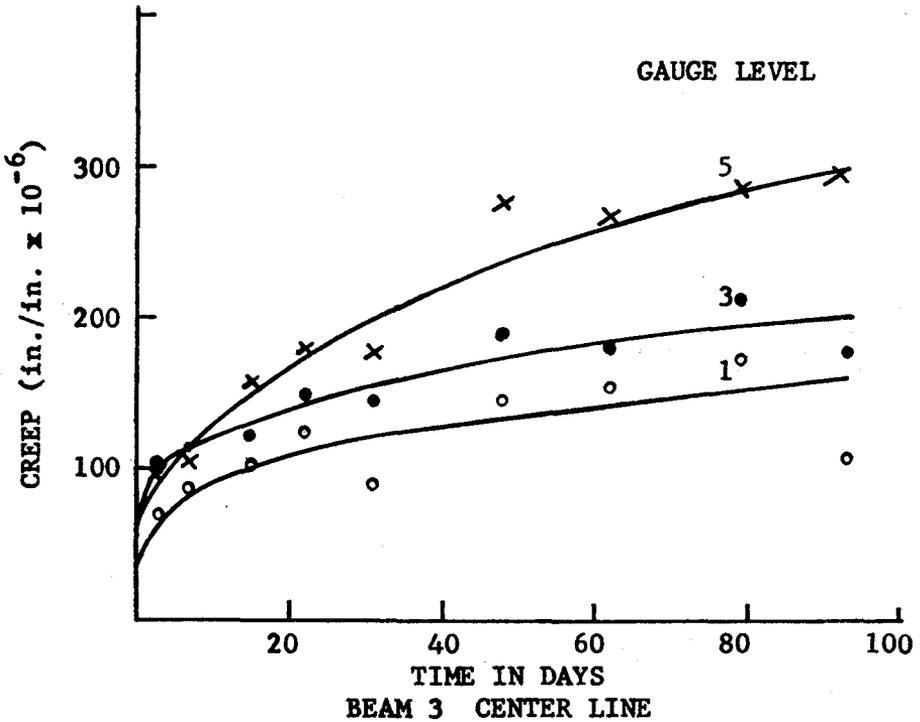
FIG. 17 - CONCRETE CREEP CURVES, BEAM 3
