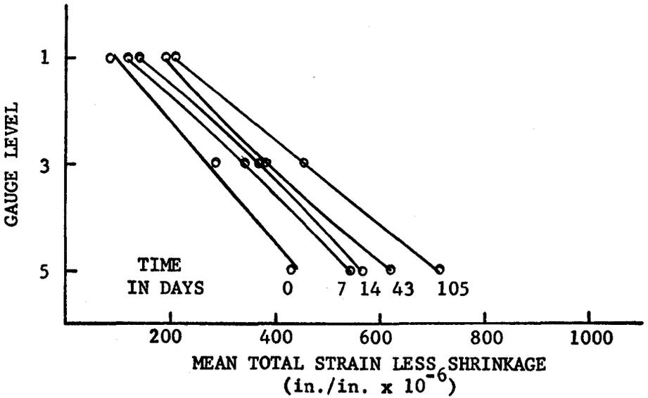
FIG. 11 - CONCRETE STRAIN DISTRIBUTION, BEAM 1, NEAR END
