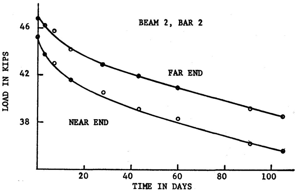
**FIG. 5 - POST-TENSIONING FORCES, BEAM 2**
