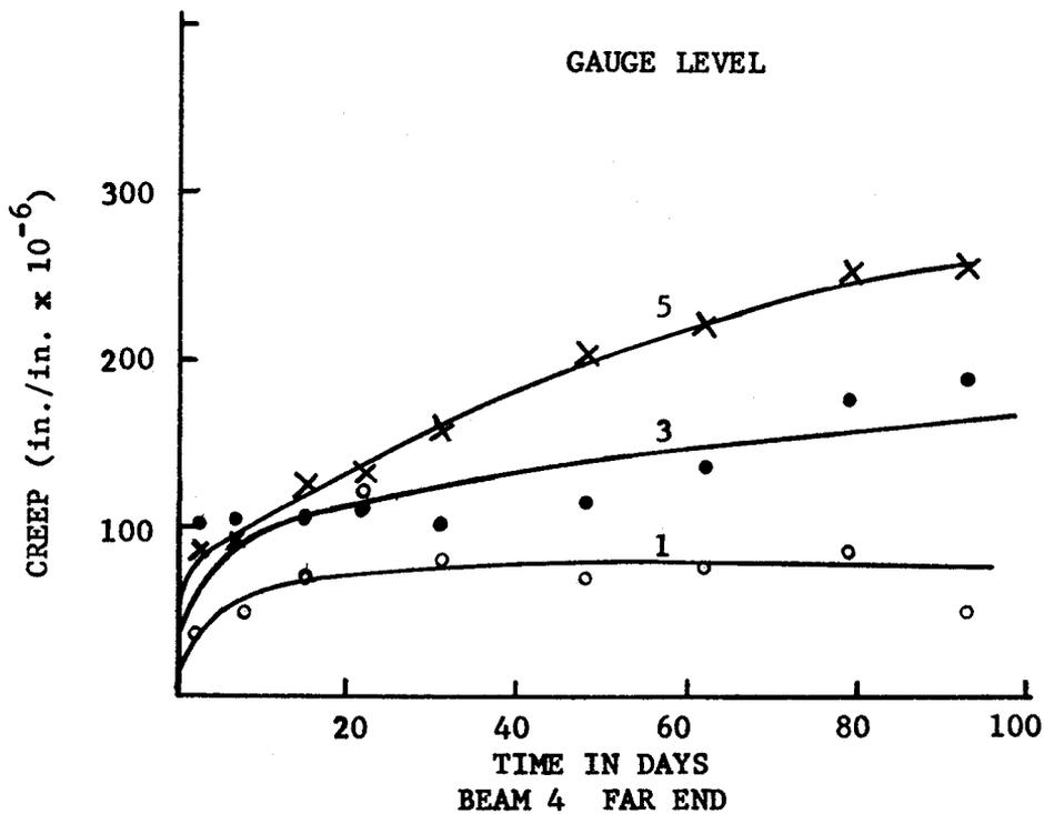
FIG. 19 - CONCRETE CREEP CURVES, BEAM 4
