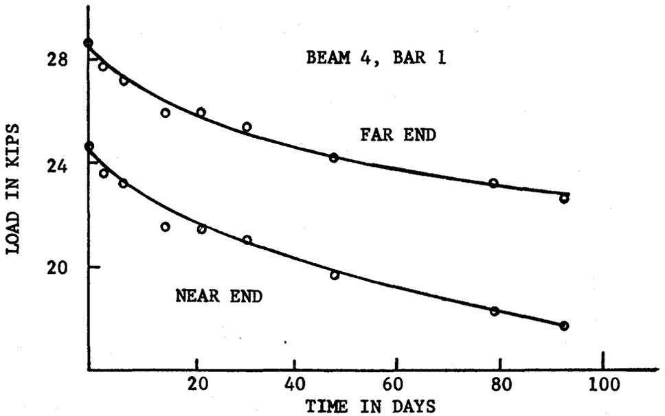
**FIG. 6 - POST-TENSIONING FORCES, BEAMS 2 AND 4**
