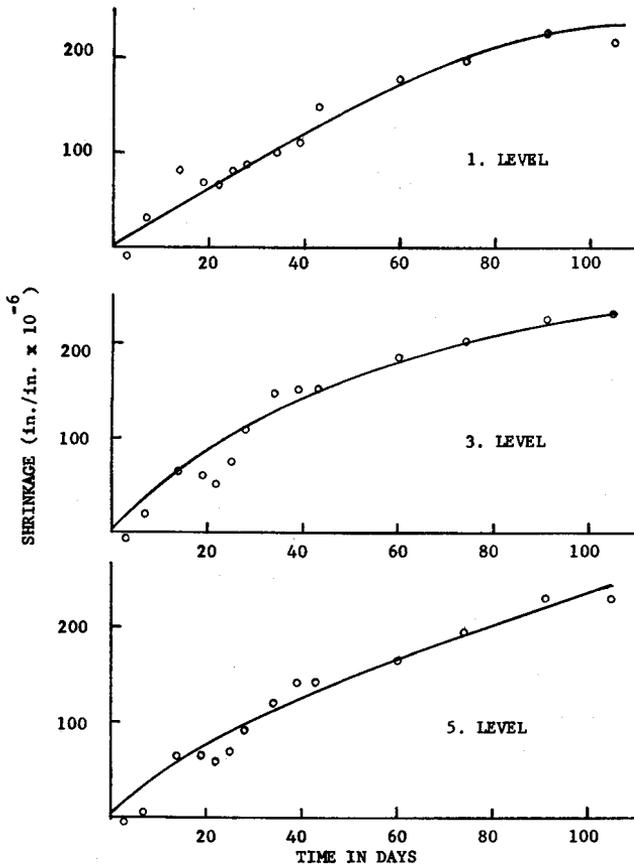
FIG. 13 - CONCRETE SHRINKAGE CURVES
