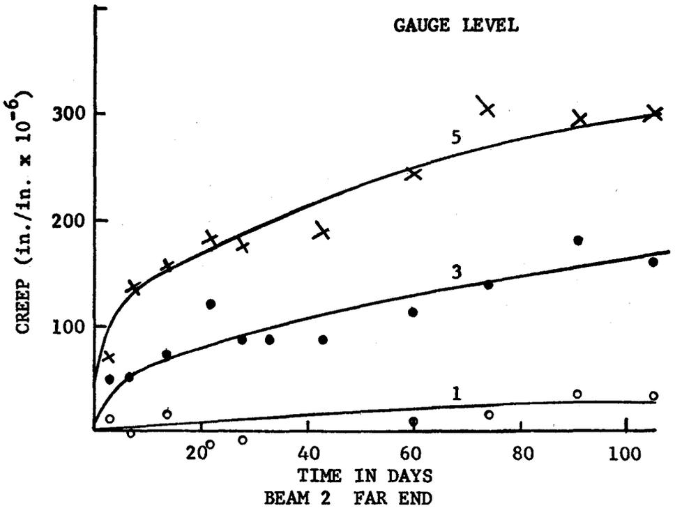
FIG. 16 - CONCRETE CREEP CURVES, BEAM 2
