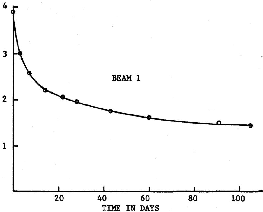
APPARENT MODULUS OF ELASTICITY
