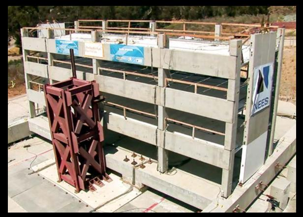
DSDM TEST BUILDING One-half scale test building shake table at the University of California–San Diego. Photo: PCI.
