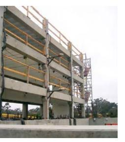
DSDM TESTING One half scale double tees and hollow-core slab. Photo: PCI.
