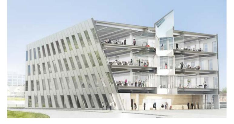
This cutaway shows how the office space adapts to the curving façade. Photo: Bjarke Ingels Group.
