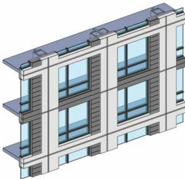
Figure 1b Typical precast panel elevation.
