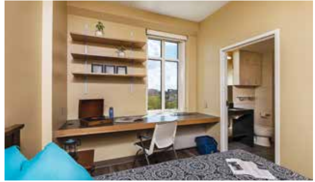
Each single-occupancy bedroom in the suites includes its own bathroom, which was slid into place as a unit.
