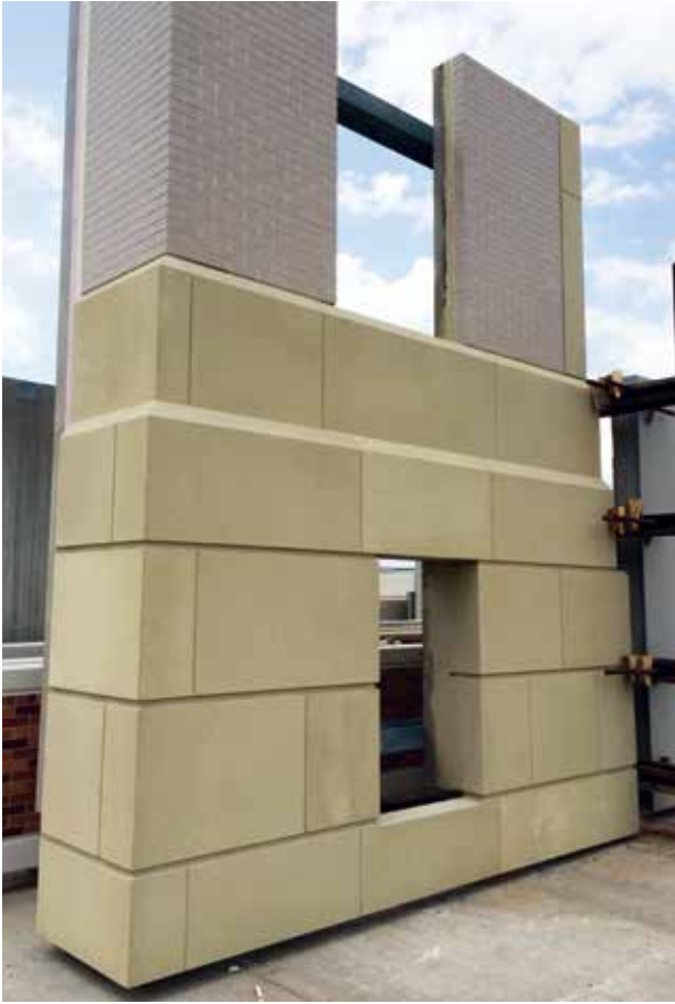
Because of the new veining technique used, a variety of mock-ups, from small samples to full-scale panels with windows installed, were created and approved.
