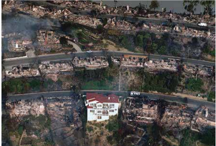
Topography, vegetation, and drought contribute to the potential for devastating wildfires. In this photo, only the concrete structure remains. Photo: Concrete Masonry Association of California and Nevada.
