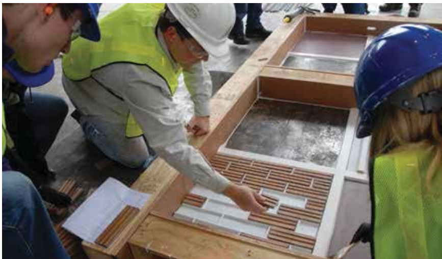
Students in the program see every aspect of precast concrete production during their plant tours. Here, they learn how to fabricate 4- x 4-foot insulated panels with four distinct finishes—thin brick, formliner, sandblast, and retarded finishes.
