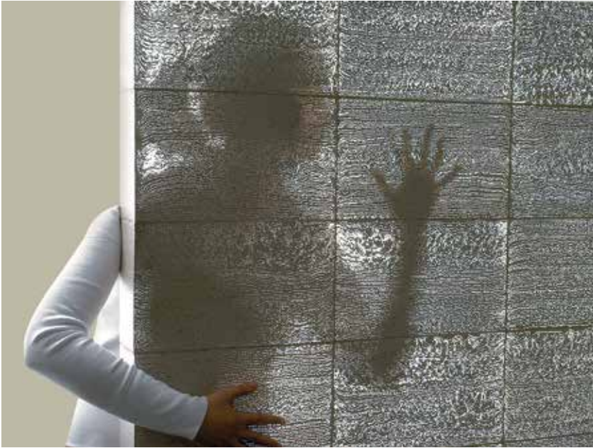
LiTraCon, based in Hungary, has created a translucent concrete consisting of concrete and glass fibers that allows opaque light to pass through, revealing shadows and shapes on the other side behind a strong light.
