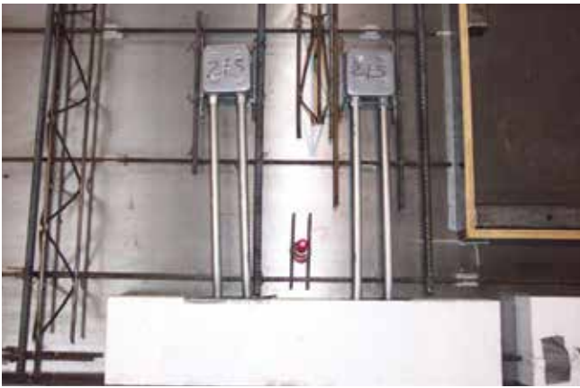
Often TPS incorporate part of the MEP systems such as electrical conduit, ductwork, or radiant heat into the panels and elements helping to save time and reduce work onsite. Photos credit: Image provided by Dukane Precast
