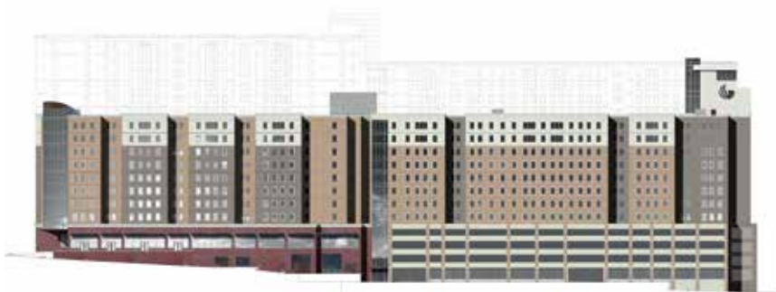
The building sits on a four-story cast-in-place parking structure on a sloping grade. The general contractor worked closely with the precaster to ensure the foundations matched perfectly, allowing the walls to be erected quickly.
