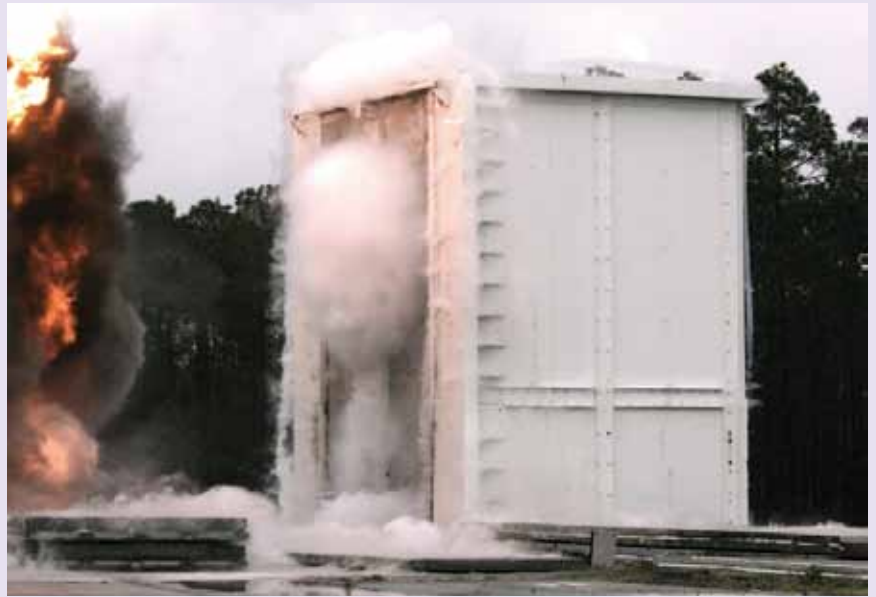
Recent tests by the Air Force Research Laboratory on precast, prestressed sandwich wall products will help determine the blast resilience of conventional off-the-shelf insulated concrete sandwich wall construction. Visit our website at www.pci.org/education/resources/index.cfm to view the video.
