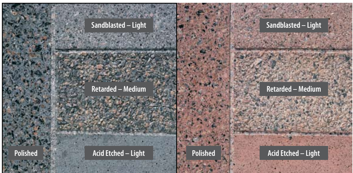
Figure 1 Appearance variations are achieved with different finishes on the same concrete mixture. (Courtesy Architectural Precast Concrete)
