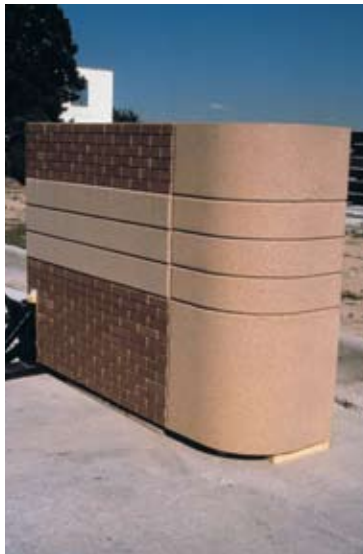
Figure 4 Panels assist in finish selection. (Courtesy Architectural Precast Concrete)
