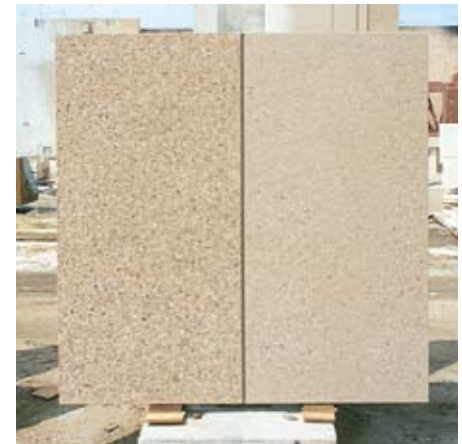
Figure 5 These range samples show retarded finishes on the left and acid-etched finishes on the right.
