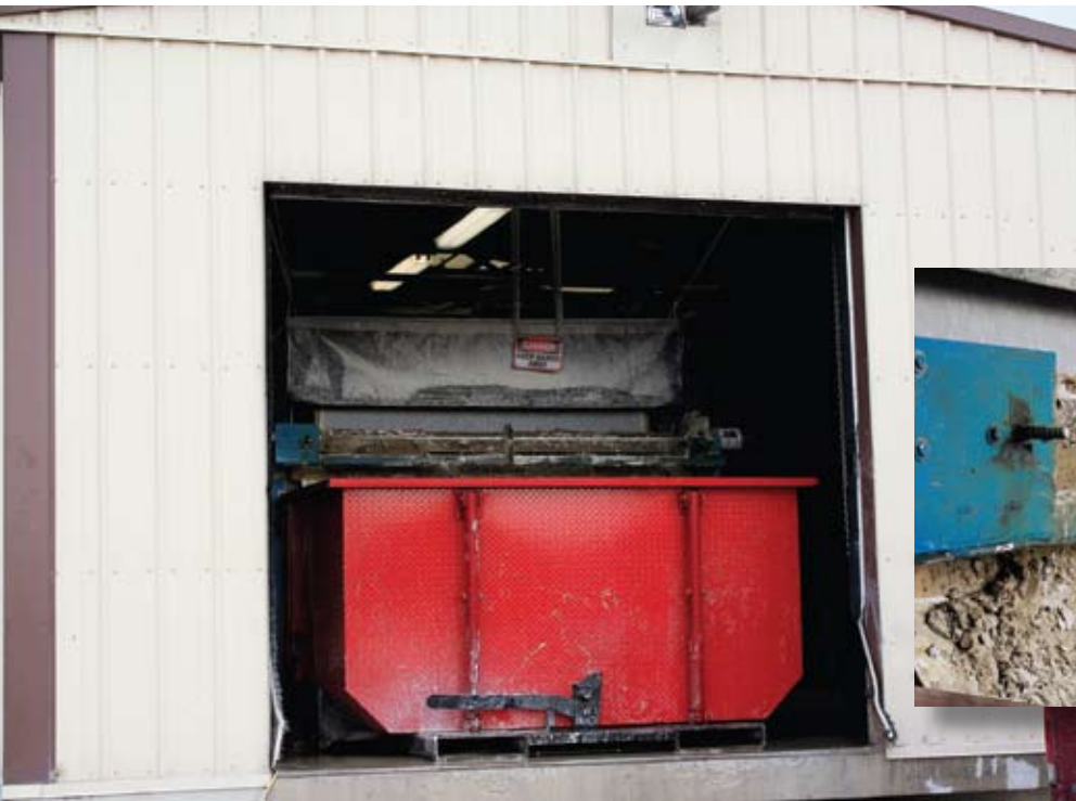
At High Concrete's plant, cement is removed by a vacuum-filtration process. The cement particles accumulate on the exterior of a rotating drum pre-coated with a layer of diatomaceous earth. The blade slices the cement off the drum, and it accumulates in a nearby hopper.
