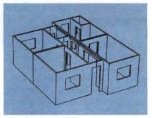
Fig. 8B. Cutaway view of assembled modules shows how extensions cast with the boxes permit enclosing a portion of the central corridor to create a bathroom.
