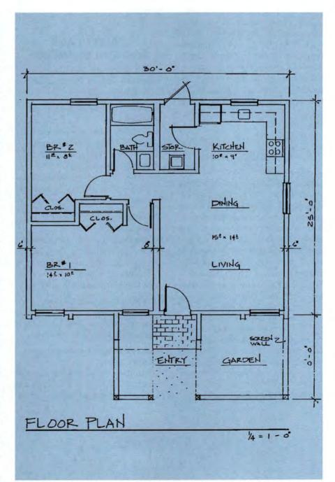
Fig. 10D. Floor plan of small residence designed with a single panel comprising each of the four basic exterior walls.
