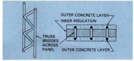
Fig. 10C. Cross section of laminated panel.
