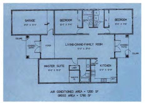
Fig. 7F. Floor plan for 1500 sq ft (140 m<sup>2</sup>) home shows how two 13x40 ft (4x12 m) modules are aligned with an offset, and spaced 13 ft (4 m) apart. The gap between is spanned by the precast concrete roof. A block-off in the standard form enabled casting a half module for the garage addition.
