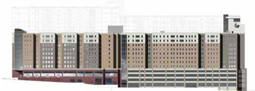
*The building sits on a four-story cast-in-place parking structure on a sloping grade. The general contractor worked closely with the precaster to ensure the foundations matched perfectly, allowing the walls to be erected quickly.*
