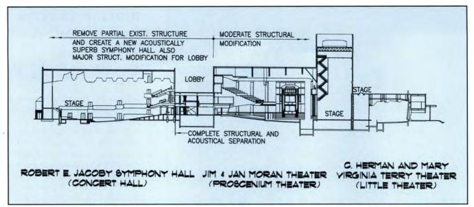
Fig. 7. Longitudinal section showing the grade levels and heights for the new and old structures. Note the two balconies added to the new section at left, which cantilever off the rear wall.
