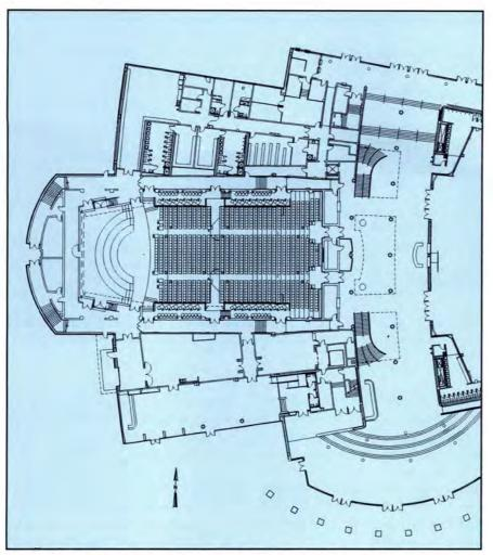
Fig. 6. The theater is designed in a long, narrow format to enhance acoustics. The new theater and office addition fits onto the original building (far right).
