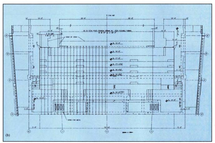
Fig. 13. Post-tensioned strand plans for the upper (top) and lower (bottom) balconies in the new theater.
