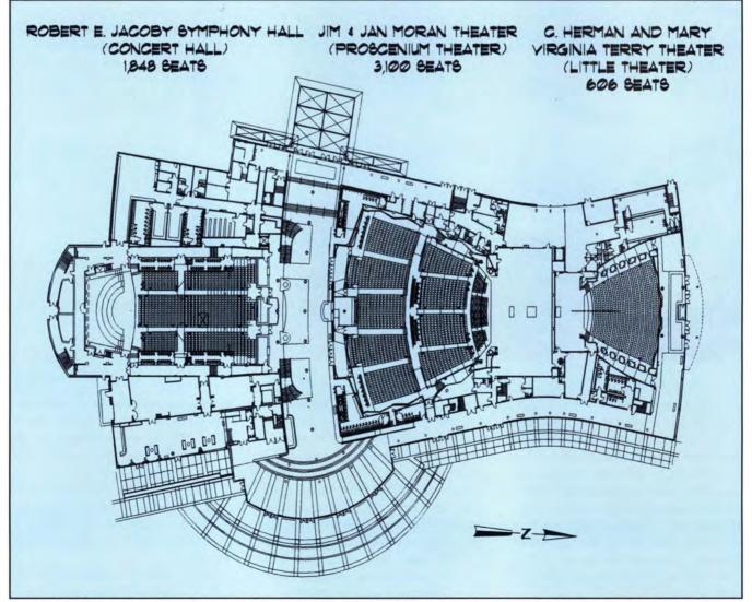
Fig. 5. Floor plan showing how the new construction (left) connects to the existing building. The structure was removed in the lobby of the Moran Theater (center) with new construction added to the left.
