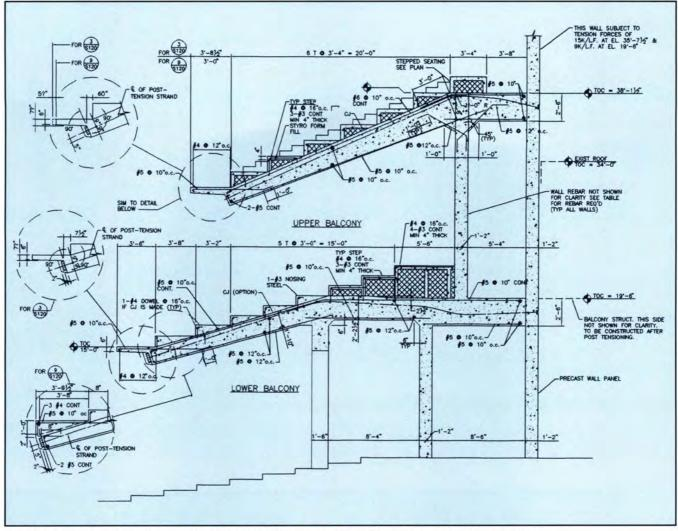
Fig. 11. Sectional drawing showing how the balconies were cantilevered off the rear wall of the theater.
