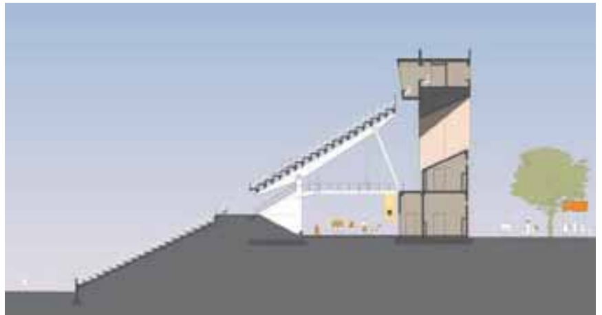
The precast concrete risers making up the top portion seem to “float” over the cast-in-place bowl seating due to their support on cast-in-place piers and precast concrete wing beams on the bottom and steel posts connecting to the precast concrete building panels at the top.
