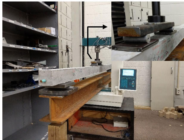
Figure 6: Overall View of Load-Displacement Test Setup
