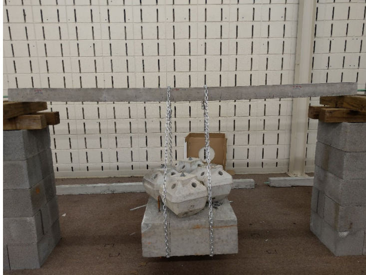
Figure 3: Picture of Sustained Load Setup
