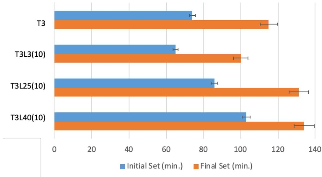
**Fig. 3: Vicat time of set for Type III cement and limestone blended cements**
