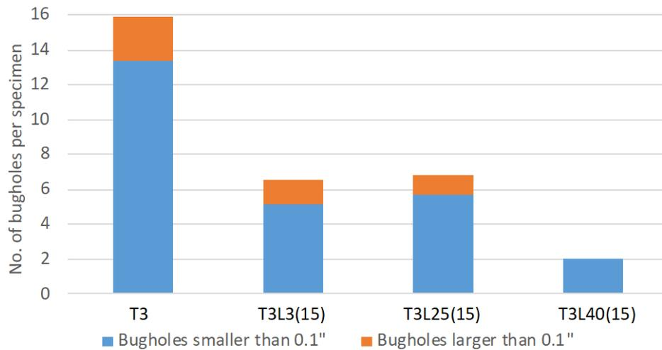
**Fig. 5: Surface finish of concrete mixes with varying limestone blended cements**
