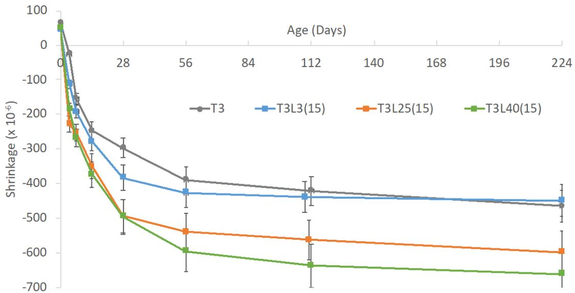
**Fig. 7: Drying shrinkage of concrete prisms cured for 24 hours and allowed to air dry**
