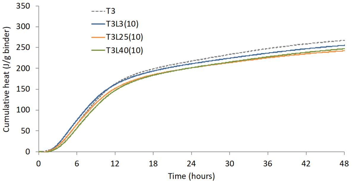
**Fig. 2: Heat of hydration curve (above) and cumulative heat (below) of Type III cement and limestone blended cements**
