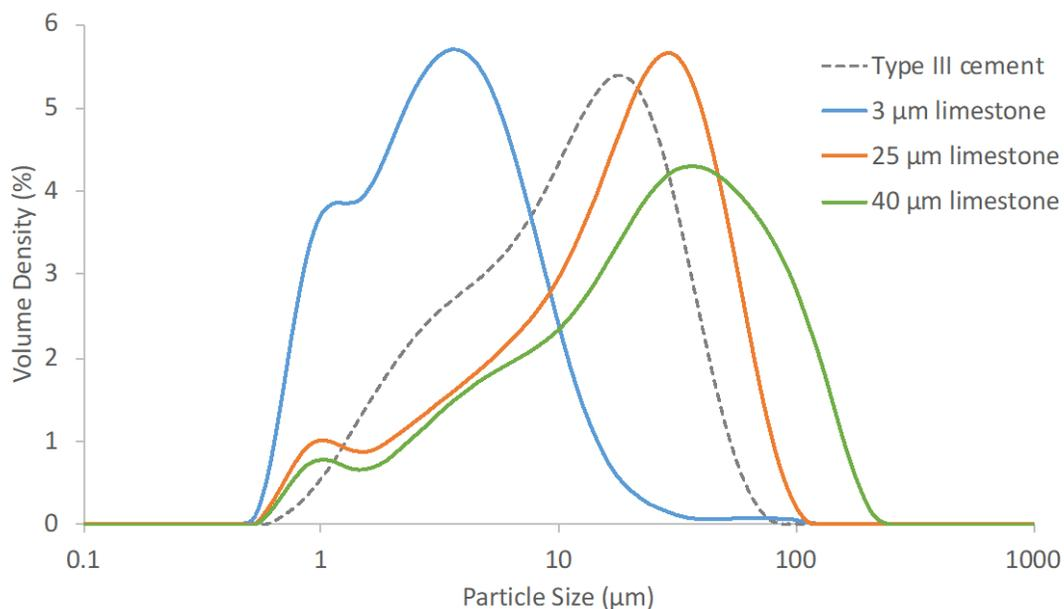
**Fig. 1: Particle Size Distribution of Type III Cement and Limestone Powder**
