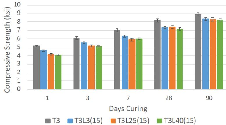
**Fig. 6: Compressive strength of Type III cement and limestone blended cements**
