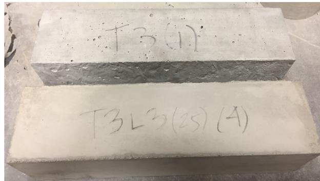
**Fig. 4: Surface finish of concrete without (top) and with limestone powder (bottom)**
