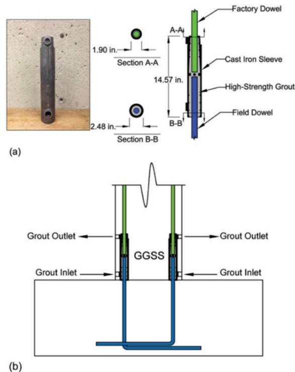
Figure 1: Grouted splice sleeve connection located in plastic hinge of the column<sup>4</sup>
