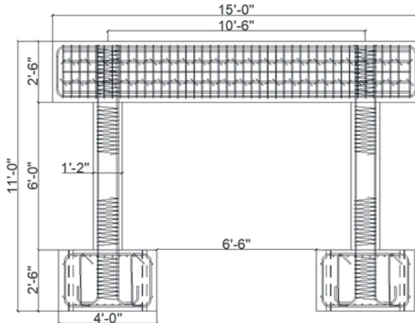
**Figure 3: Cast-in-place bent benchmark details**
