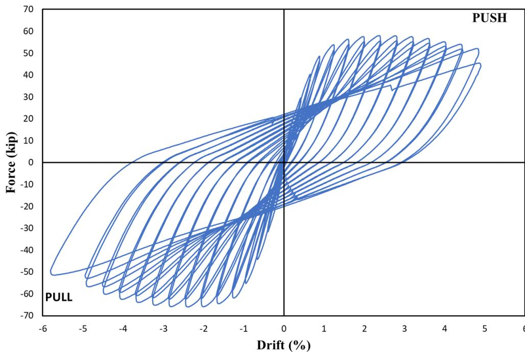
(a) Cast-in-place bent
