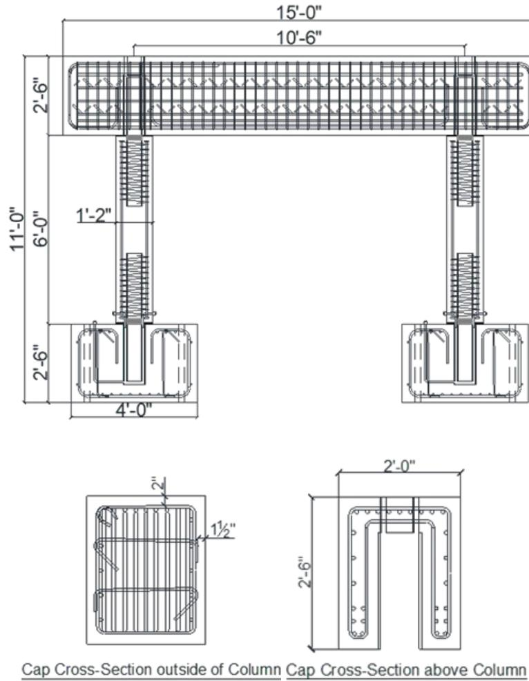
**Figure 4: Precast bent details**
