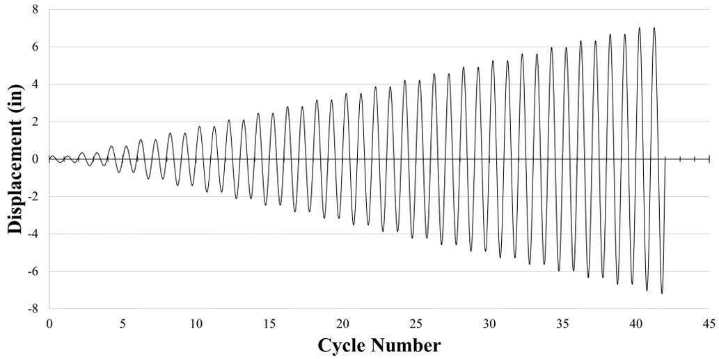
Figure 5: Quasi-static loading protocol
