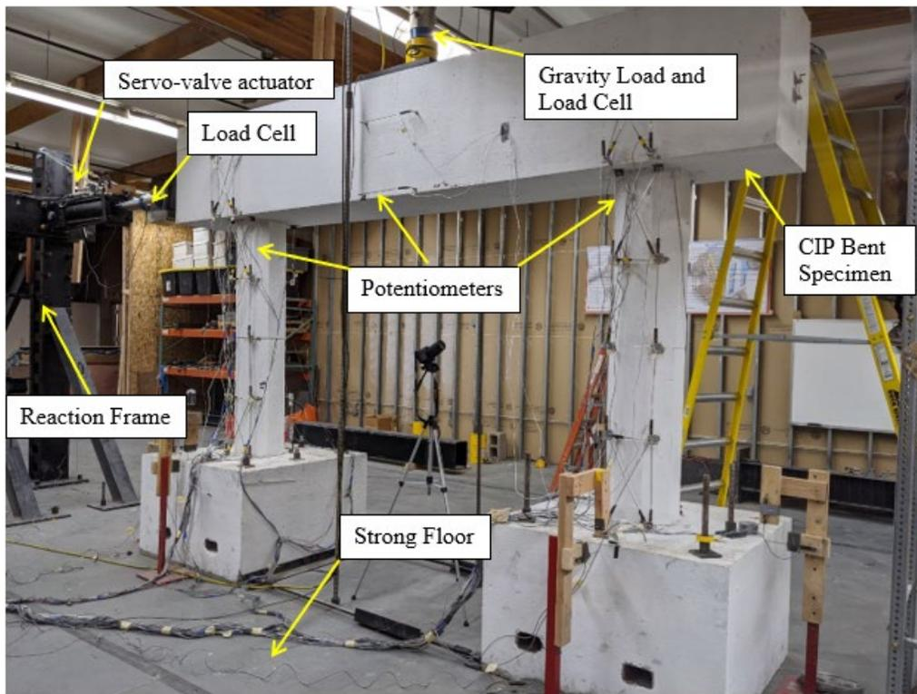
Figure 6: Bent Testing Arrangement
