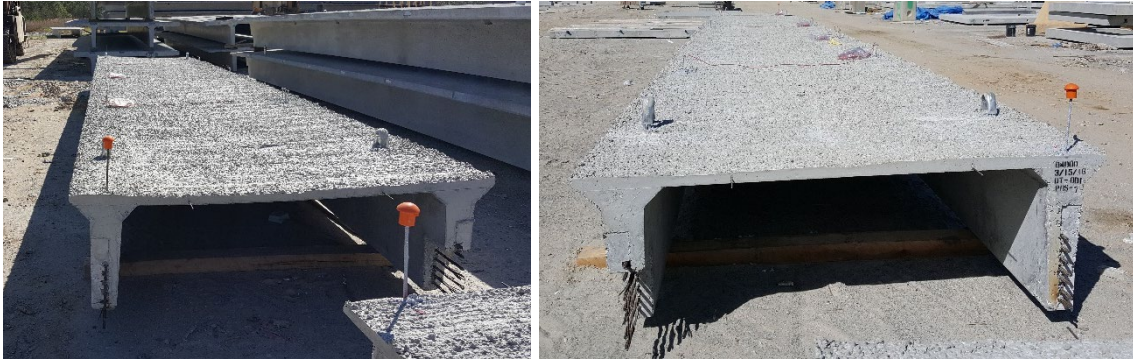
Figure 6 – 40ft and 60ft test specimens on dunnage for storage
