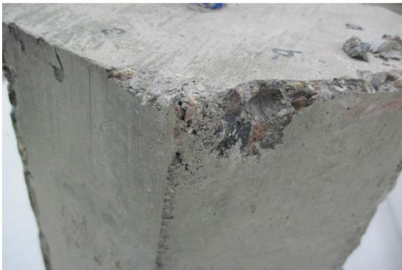
Fig. 14 Specimen 22Sp2 crushing on live end
