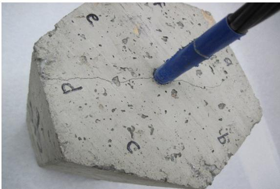
Fig. 18 Specimen 1St2 cracking on live end
