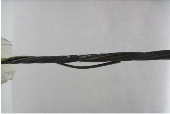
Fig. 13 Specimen 4Sp2 failure due to strand breaking
