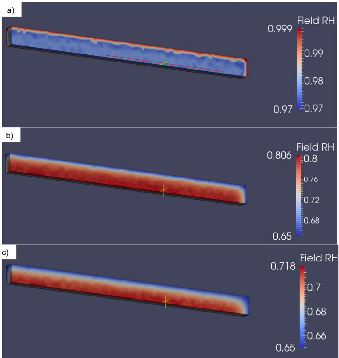
Figure 9: The evolution of RH gradient with time inside full-scale beam at: a) 2 days, b) 100 days, and c) 400 days.
