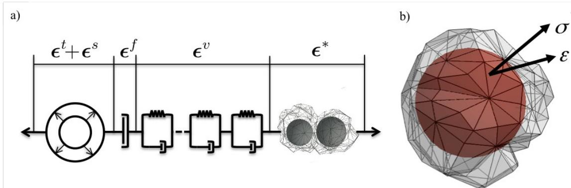
Figure 1: a) Equivalent rheological model based on strain additivity, b) One LDPM Cell around an aggregate piece with facet stress and strain vector
