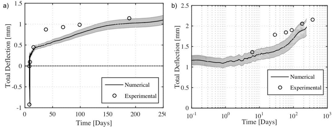
Figure 10: a) Total beam deflection from casting, b) long term beam deflection measured from loading.
