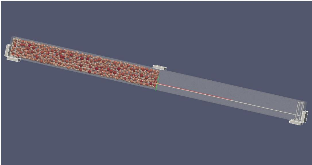
Figure 4: Coarse LPDM mesh for full-scale beam.
