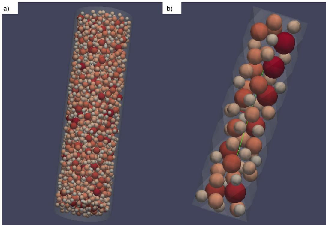
Figure 2: a) Fine LPDM mesh with minimum aggregate size of 5 mm, b) Coarse LPDM mesh with minimum aggregate size of 15 mm
