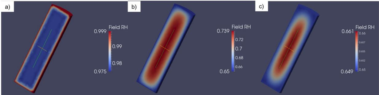
Figure 3: The evolution of RH gradient with time for 65% cylinders at: a) 2 days, b) 100 days, and c) 400 days.
