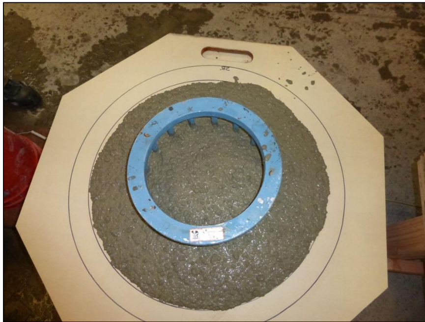
Fig. 7 Slump Flow Testing of High Performance SCC Mix Design
