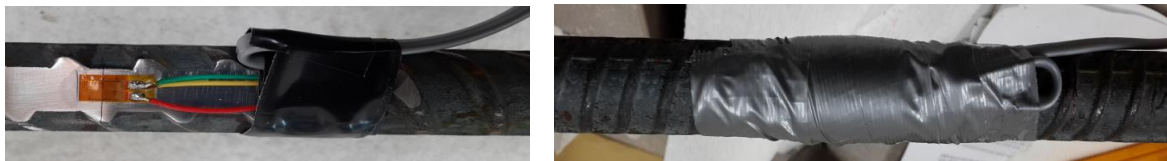
Fig. 5 Strain gage on re-bar before (left) and after (right) protective layers
