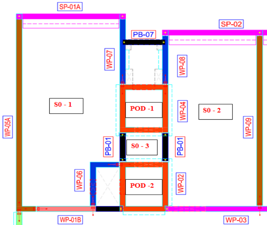
Fig. 6 Pragati Towers - Precast Panel Layout for the Typical Apartment Floor Plan
