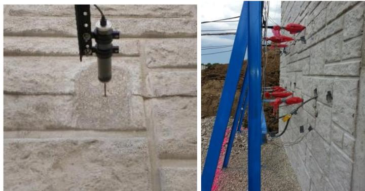
Fig. 11 Strain gauge and LVDT on concrete surface
