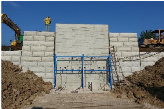
Fig.3 Front elevation TPCCRW with wing walls
