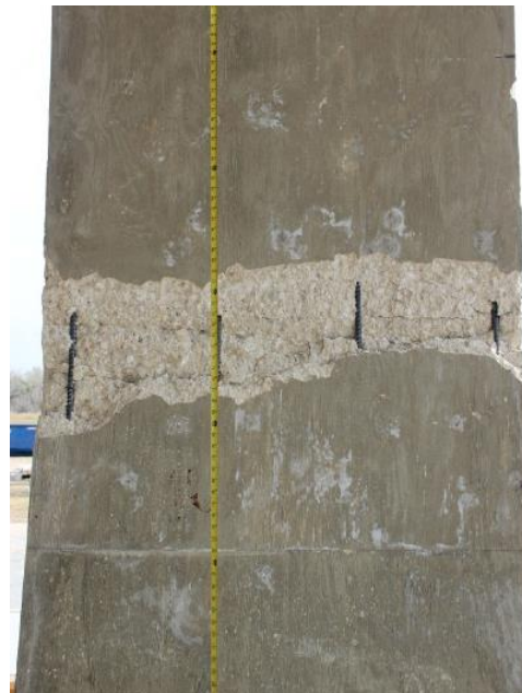
(b) Panel 3B – No shear stirrups
