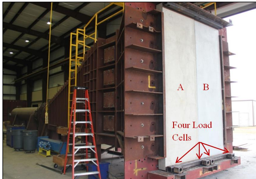
Fig. 3 Wall Specimens Mounted in Shock Tube
