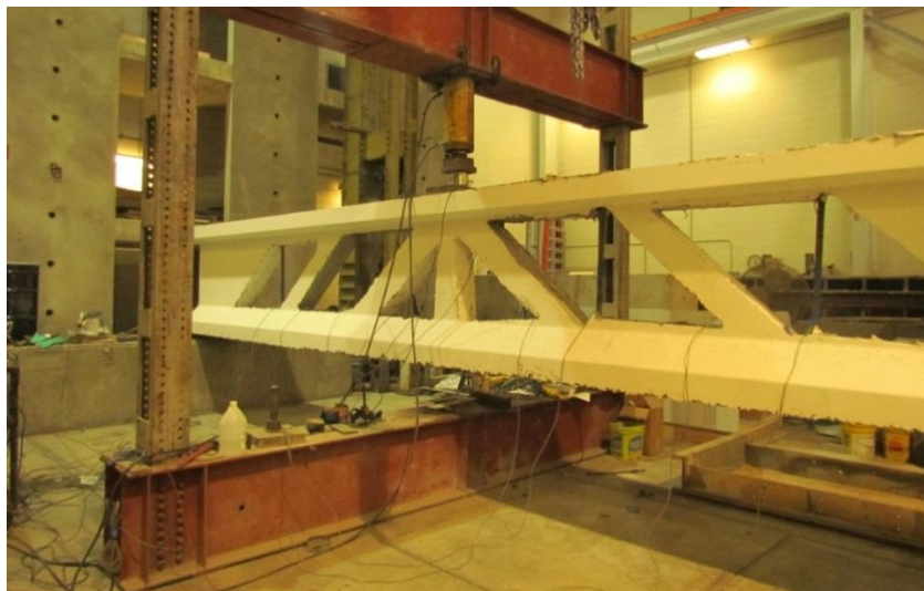
Fig. 16 Instrumented truss specimen during loading
