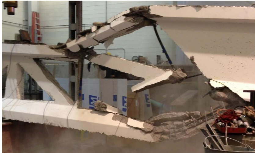
Fig. 137 Failure of the truss specimen
